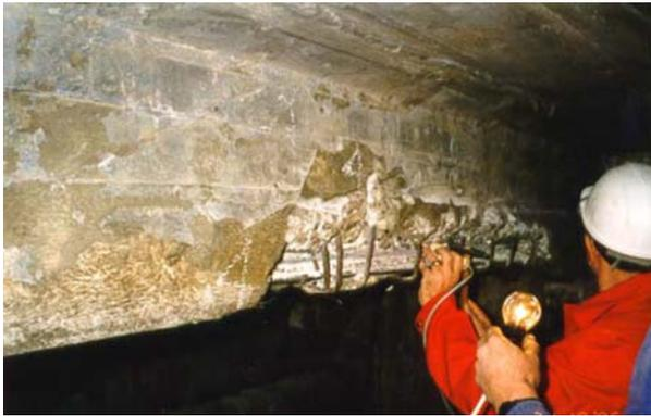
**Figure 5.1.** In situ measurement of actual prestressing force with steel-bar vibration frequency recording
