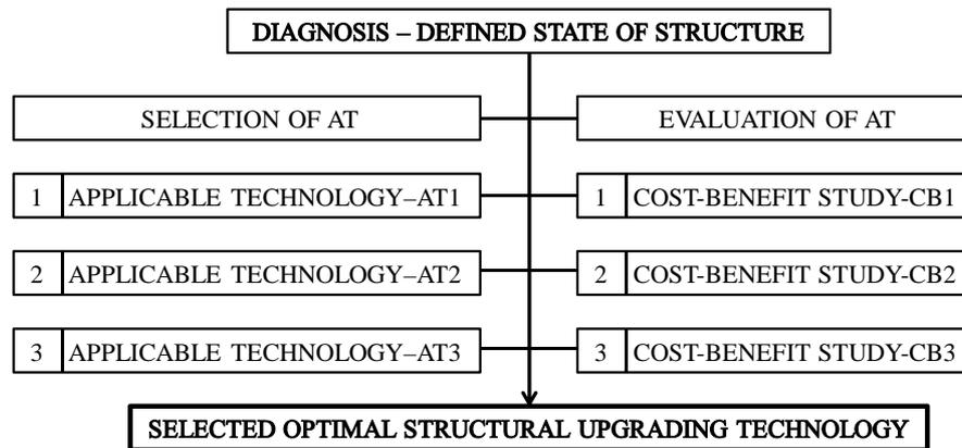
**Figure 4.1.** Advanced CB-Method for selection of optimal common and/or seismic upgrading technology
