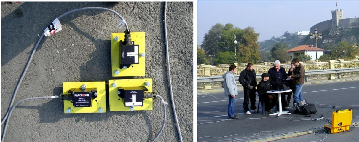
**Figure 5.10.** Realization of the second ambient vibration tests of the unique twin-city bridge “Goce Delcev” in Skopje after the completed revitalization project: (1) Installation of 3-componental DIGITEXX sensors and (b) Part of project team preparing the testing procedure and permanent data acquisition unit
