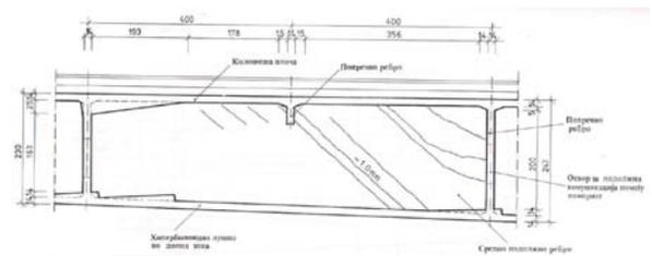
**Figure 5.6.** Downstream bridge: Detail of identical cracks along RC longitudinal superstructure beam
