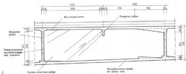
**Figure 5.5.** Upstream bridge: Detail of recorded inclined open cracks along RC longitudinal superstructure beam
