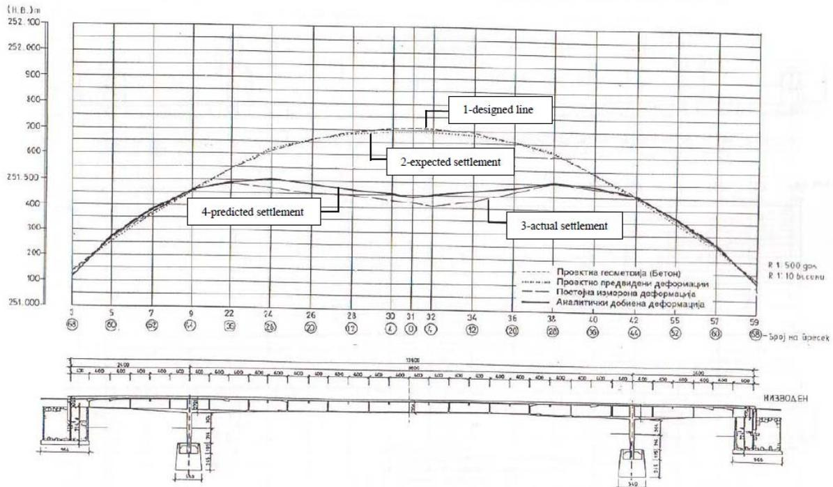
**Figure 5.8.** Upstream bridge: Longitudinal distribution of large settlements of the complete RC bridge superstructure defined by precise geodetical measurement (comparative plot: 1-designed line; 2-expected settlement; 3-actual settlement and 4-predicted settlement by the formulated experimentally verified nonlinear analytical model).
