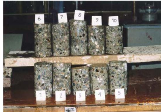
**Figure 5.2.** Determination of actual concrete strength based on compression tests on samples
