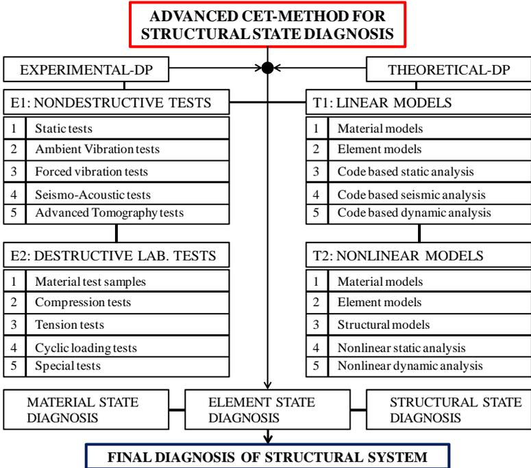
**Figure 3.1.** Advanced combined experimental and theoretical (CET) method for structural state diagnosis
