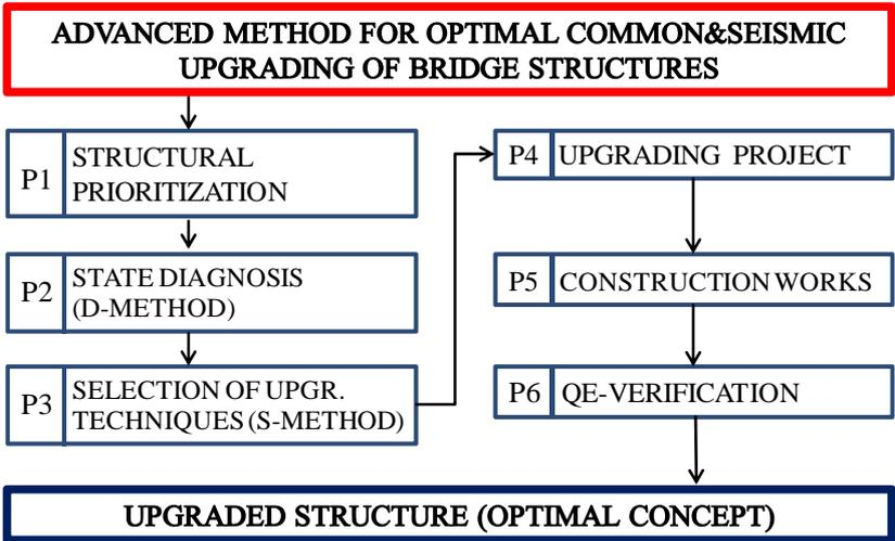
**Figure 2.1.** Advanced general concept for optimal common & seismic upgrading of bridge structures with six principal phases
