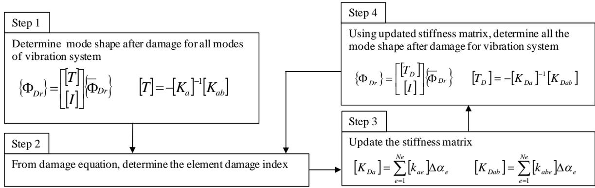
Figure 3.1. Flow chart of one cycle in damage identification using Guyan's method
