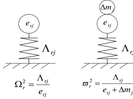
**Figure 5.2.** Principle of the mass sensitivity method
