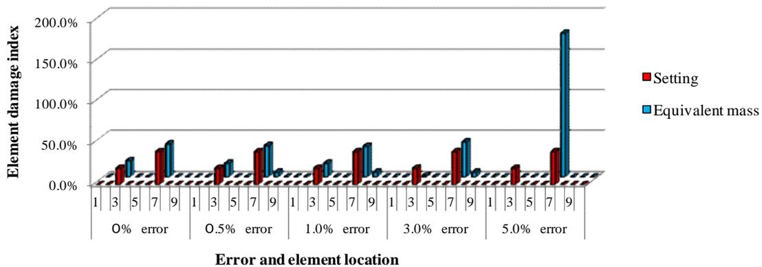
**Figure 5.4.** Results of damage identification that contain error in the equivalent mass
