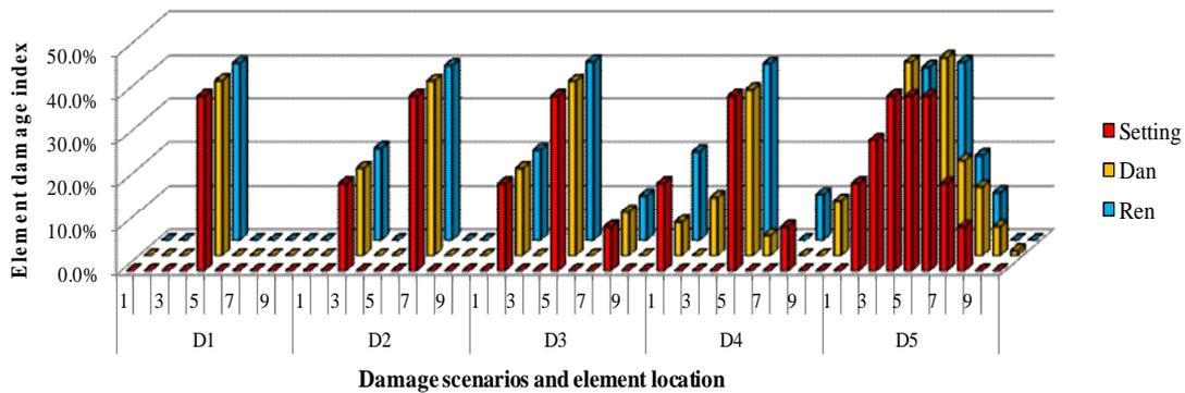
Figure 3.2. Damage identification results for scenarios D1-D5
