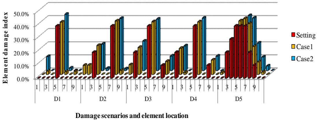
Figure 4.1. Damage identification results in case of using added mass
