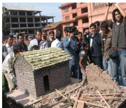
Fig 3.7 Shake table result' Non-retrofitted building collapse while retrofitted building is standing
