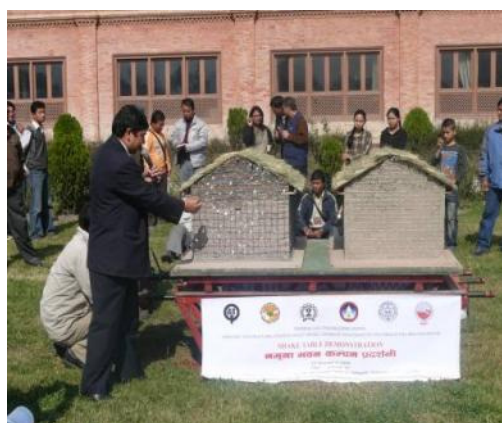
Fig 3.6 Two identical buildings with and without retrofitting by PP Band before shake table
