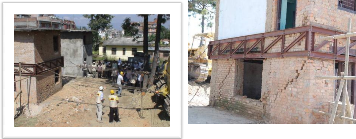
Fig 3.2 Loading arrangement (left) and crack propagation (right) during pull down test of non-retrofitted building
