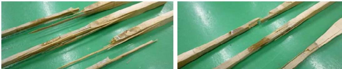
**Figure 2.7.** Fracture surface tested at 56 days: (left) w/c ratio =100%; (right) w/c ratio =80%
