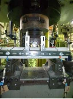
Figure 4.2. Bending test setup
