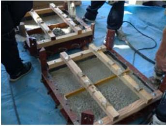
Figure 4.3. Casting of slab specimens
