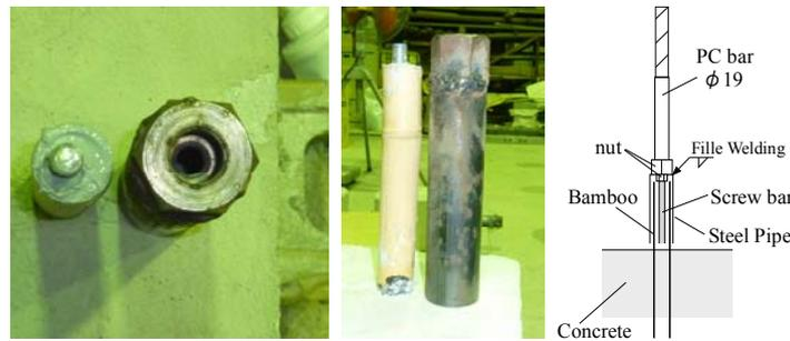
Figure 3.5. Detail of Joints between Bamboo and PC bar
