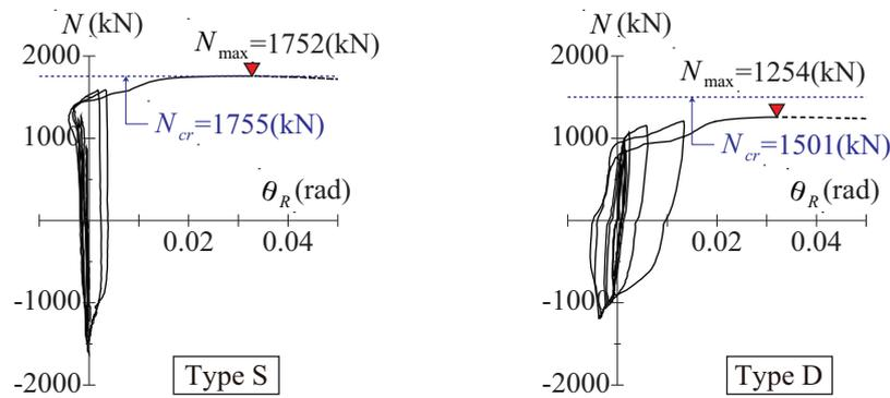
**Figure 9.** Axial force of knee brace damper versus rotational angle of brace joint relationship
