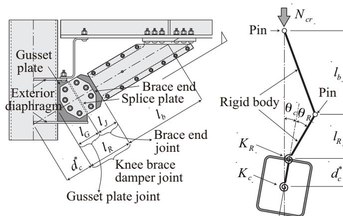
Figure 8. Buckling model
