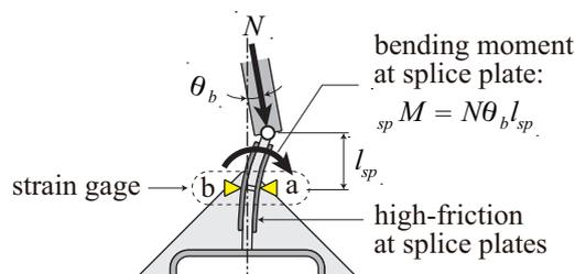
**Figure 11.** Bending moment at splice plates
