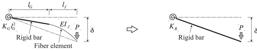
**Figure 13.** Knee brace damper joint model
