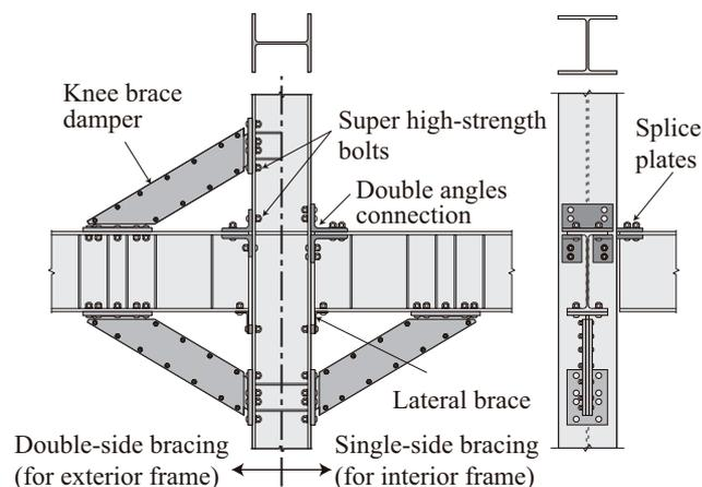
**Figure 1.** Details of weld-free system (wide-flange column)
