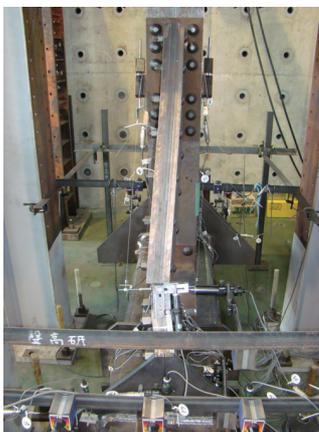
Figure 7. Out-of-plane buckling
