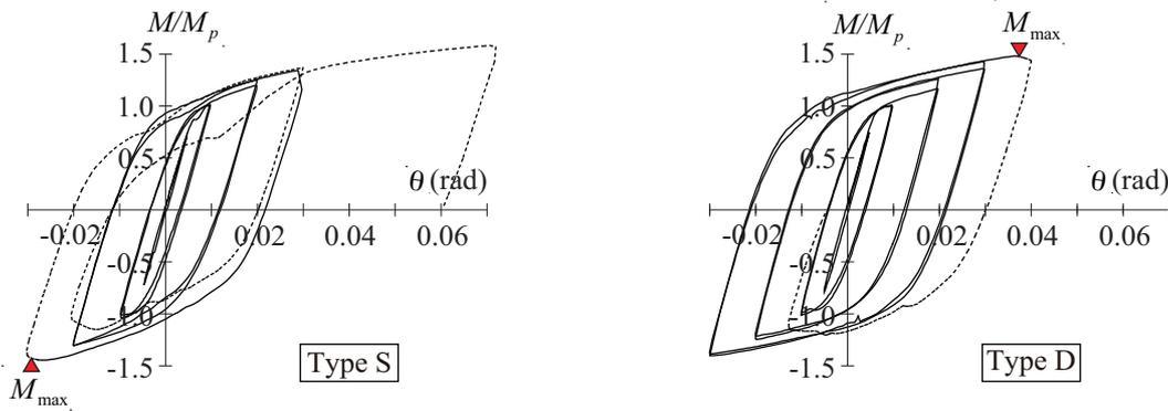
Figure 6. Bending moment at the beam end versus beam rotation angle relationship
