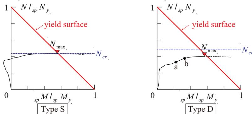
**Figure 10.**  $M$ - $N$  interaction at splice plates of knee brace damper
