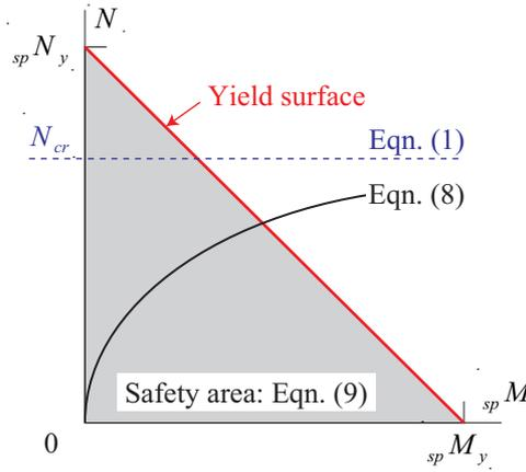
**Figure 14. Design criteria of brace joint**
