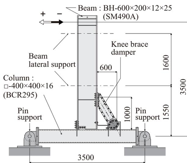
Figure 4. Test setup (unit: mm)
