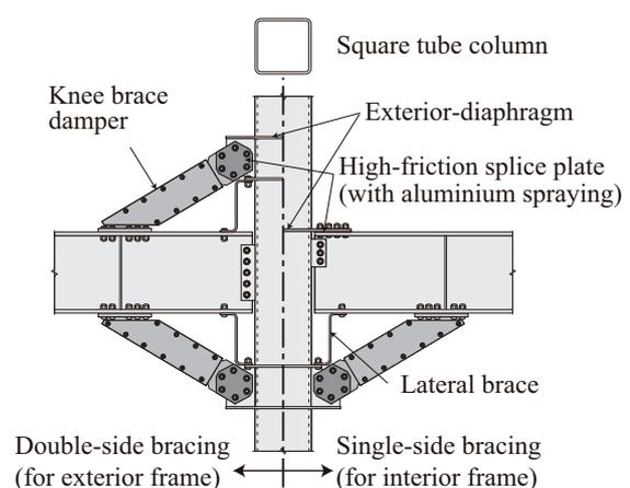
**Figure 2.** Details of weld-free system (square tube column)
