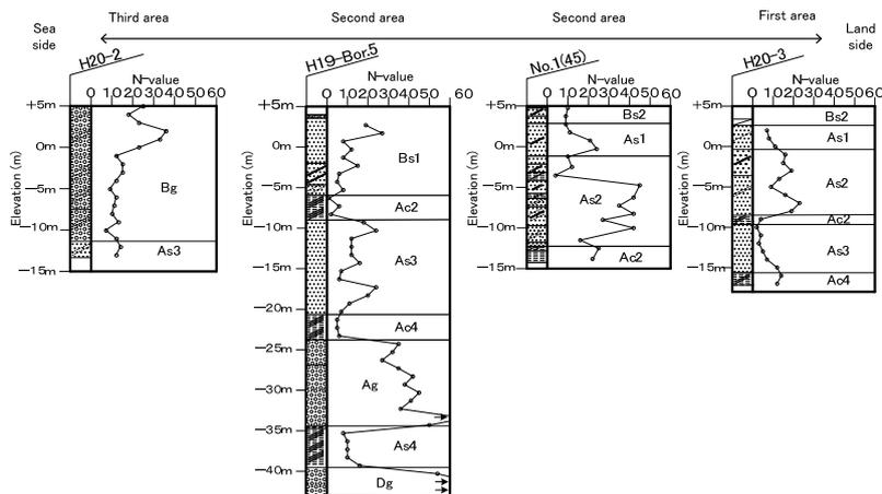
**Figure 3.2.** Existing boring logs along field survey line
