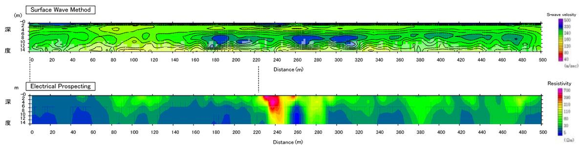
**Figure 3.7.** Results of Surface wave Method and Electrical Prospecting in Tokyo International Airport
