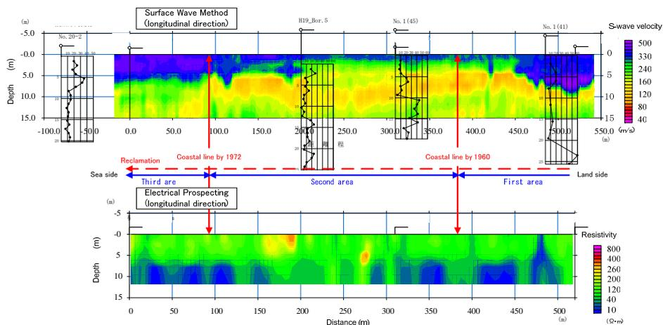
**Figure 3.3.** Results of Surface Wave Method and Electrical Prospecting in Matsuyama Airport
