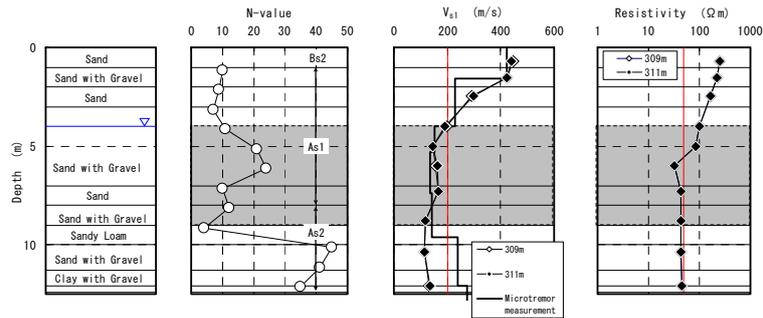
Figure 4.1. Example of distributions of S-wave velocity and resistivity
