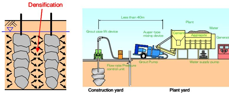
**Figure 3.6.** General use of compaction grouting
