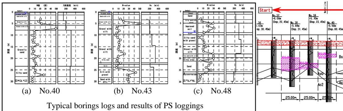
Typical borings logs and results of PS loggings
