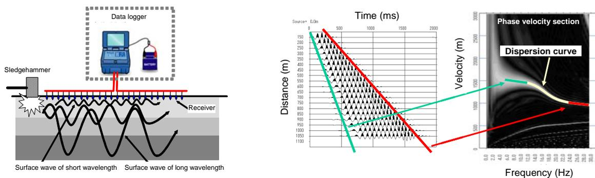
(a) Schematic view of a surface wave method
