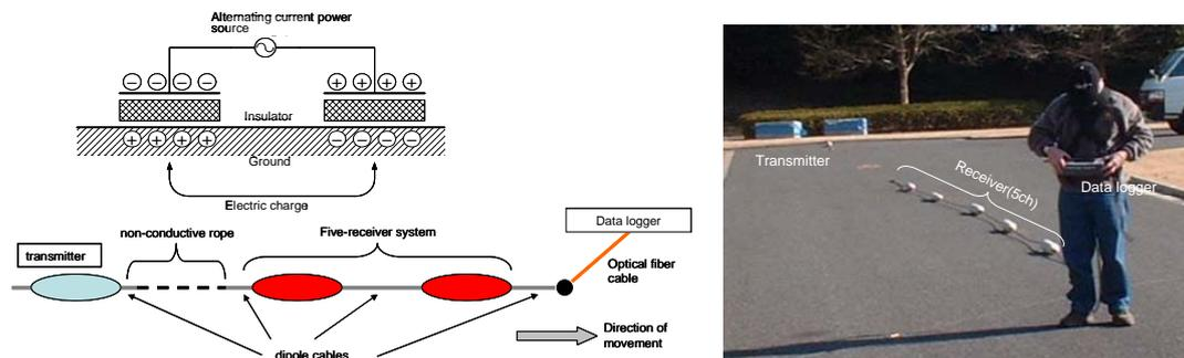
**Figure 2.2.** Concept of the capacitively-coupled resistivity measurement and the five-receiver system
