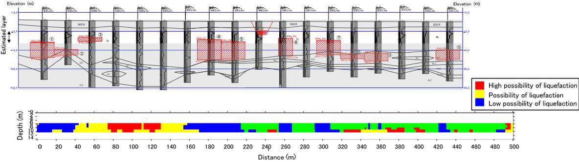
**Figure 4.4.** Estimation of liquefaction resistance in Tokyo International Airport
