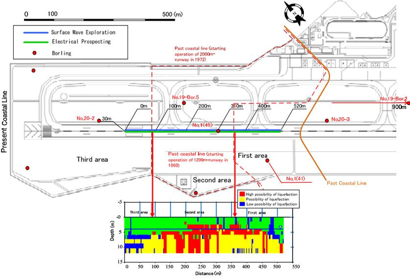
**Figure 4.3.** Estimation of liquefaction resistance in Matsuyama Airport
