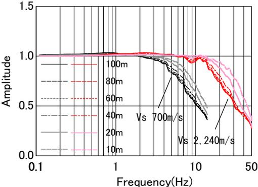
**Figure 8.** Comparison of the average transfer function on the ground surface. (Effect of soil properties and correlation distance)
