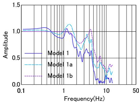
Figure 15. Transfer functions at the foundation to the surface of free field for 3 different scale of models.
