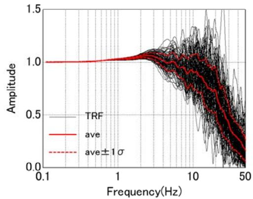
**Figure 6.** Transfer functions of the horizontal component of the foundation to the surface of free field. The average and the standard deviation of the results of MCS for B2g100 (B: model w/ foundation).
