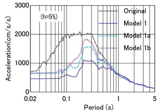
Figure 16. Acceleration response spectra at the foundation of 3 different scale of models.
