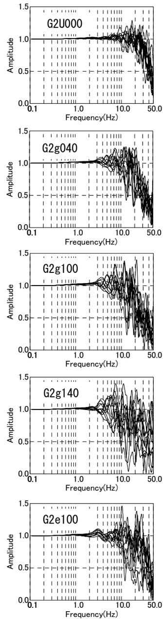
**Figure 3.** Transfer functions of the horizontal component on the ground surface against the surface of free field (H/H)
