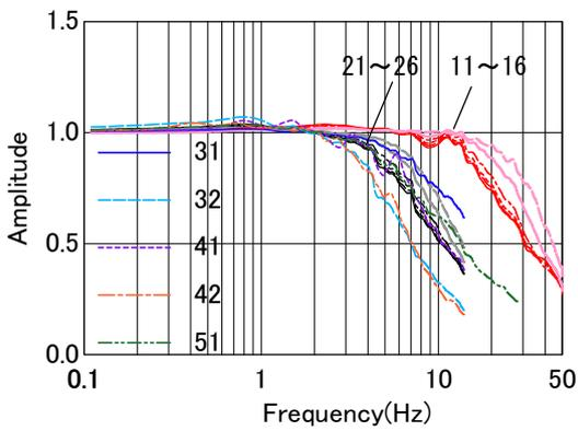
**Figure 17.** Comparison of transfer functions at the foundation to the surface of free field for all models versus frequency.
