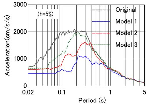
Figure 13. Acceleration response spectra at the foundation of 3 similarity models.
