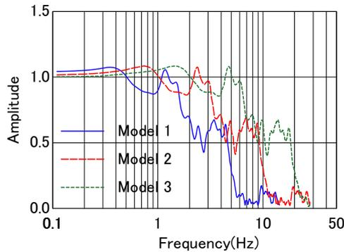
Figure 12. Transfer functions at the foundation to the surface of free field for 3 similarity models.
