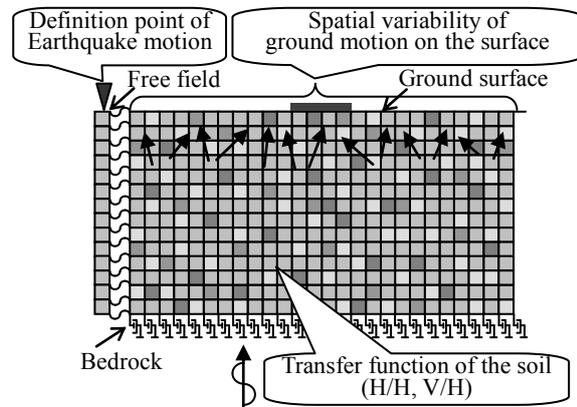
**Figure 1.** Concept of analysis and soil model
