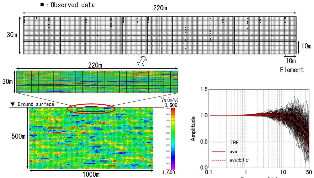
Figure 20 Data at the real site and a sample of a 2D-FE model.
