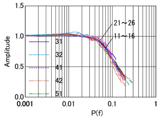
**Figure 18.** Comparison of transfer functions at the foundation to the surface of free field for all models versus heterogeneous parameter  $P(f)$ .
