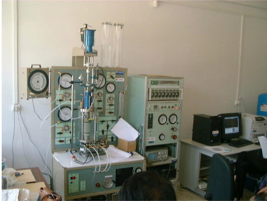
**Figure 2.1.** Triaxial Testing Apparatus Model DTC-367 by Seiken, Inc. Japan
