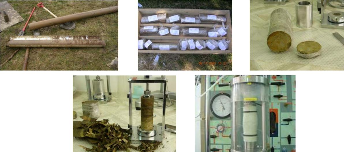
**Figure 5.2.** Sampling, preparation and testing of the soil samples
