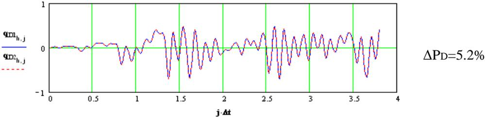
**Figure 8.** Difference of axial force between the responses of the lowest storey column in the five storey building with EBF system.
