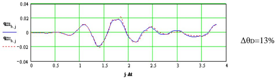
**Figure 3.** Difference of rotations between the responses of the lowest storey node in the seven storey building with MRF system.
