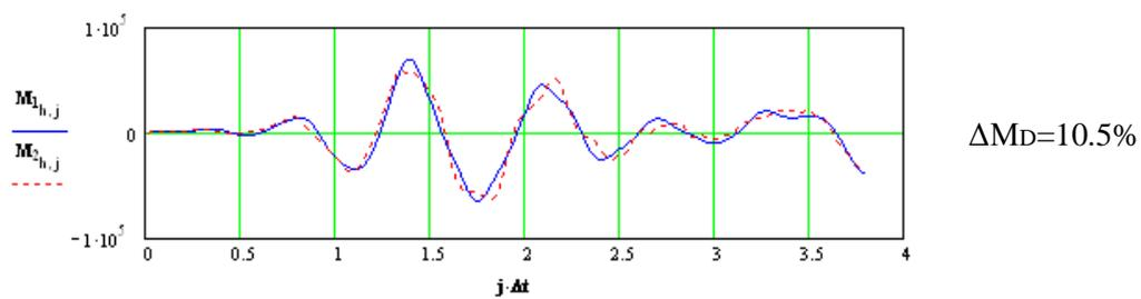
**Figure 4.** Difference of moments between the responses of the lowest storey column in the seven storey building with MRF system.
