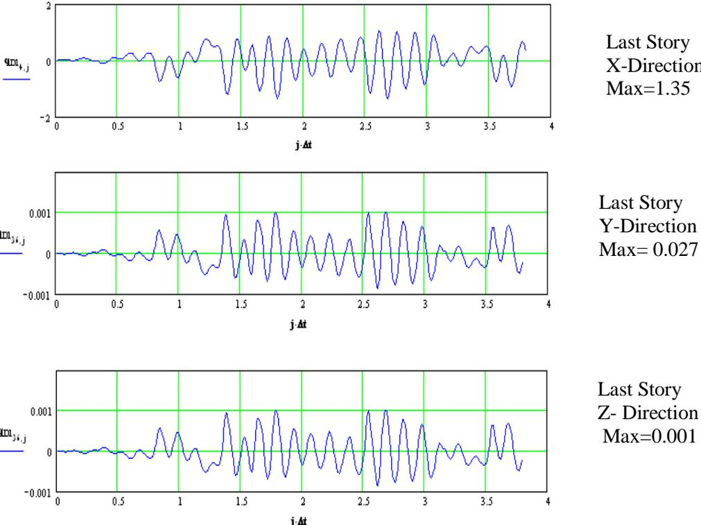
**Figure 2.** Horizontal and vertical responses and rotation of degrees of freedom in the seven storey building with EBF system.
