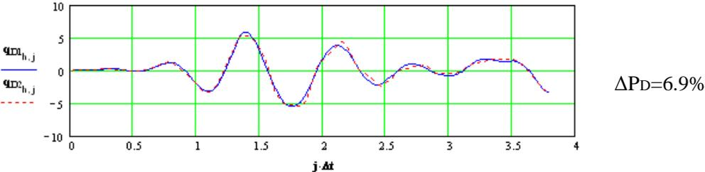
**Figure 7.** Difference of axial forces between the responses of the first and second order dynamic analyses of the lowest storey column in the five storey building with MRF system.
