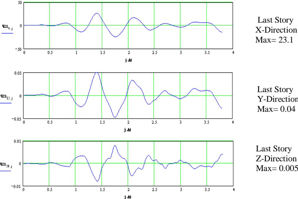
**Figure 1.** Horizontal and vertical responses and rotation of degrees of freedom in the seven storey building with MRF system.
