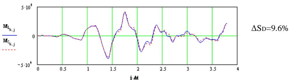
**Figure 5.** Difference of shears between the responses of the lowest storey beam in the five storey building with EBF system.
