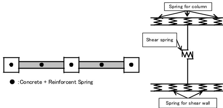
**Figure 5.** Applied analytical model
