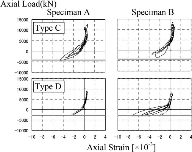
Figure 7. Relationships of axial load and axial strain
