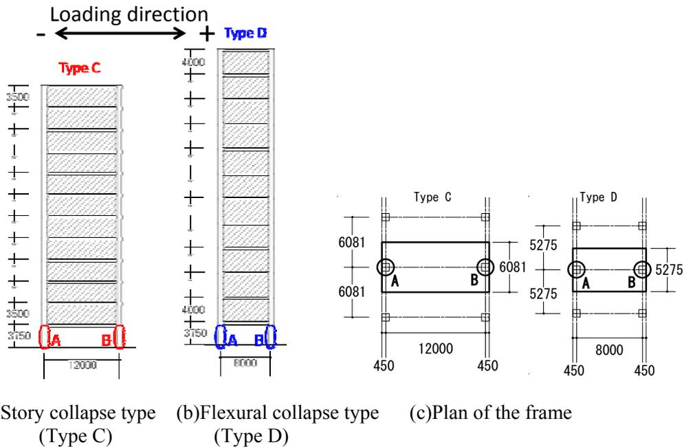
**Figure 2.** Outlines of model frames [mm]
