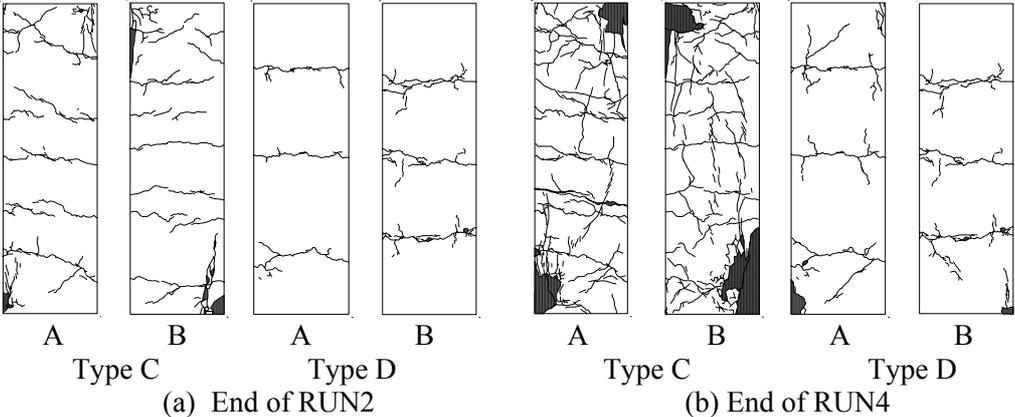
**Figure 9.** Crack patterns of specimen after test
