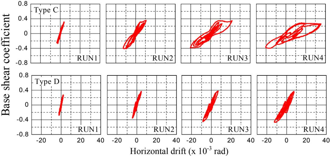
Figure 6. Relationships between base shear coefficient and horizontal drift
