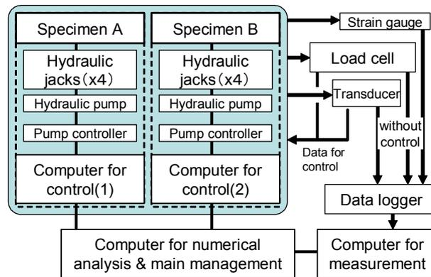
Figure 4. Outline of the substructure pseudo-dynamic test system
