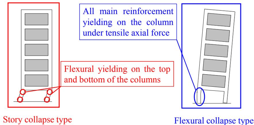
**Figure 1.** Outline of the failure modes of the soft story buildings
