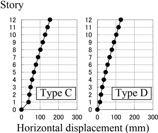
**Figure 8.** Maximum horizontal displacement of each story (RUN2)
