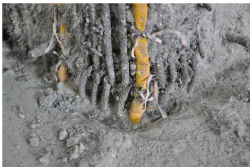
**Photo 6.** Damage in the Plastic Hinge Region after Seismic Response Loading Experiment
