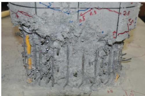
**Photo 4.** Damage in the Plastic Hinge Region after Cyclic Loading Experiment
