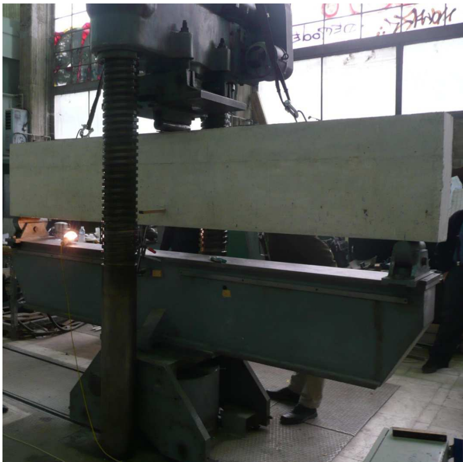
Figure 2.4. Loading of one of the specimens
