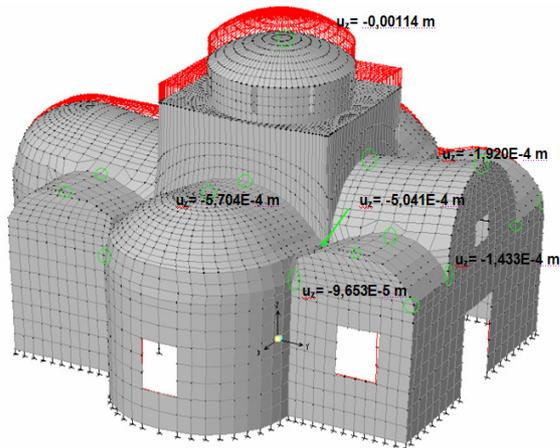
**Figure 14a.** Deformations for the Gravitational Loads  $\delta_{\max} = 1.14\text{mm}$  at the top of the central dome.
