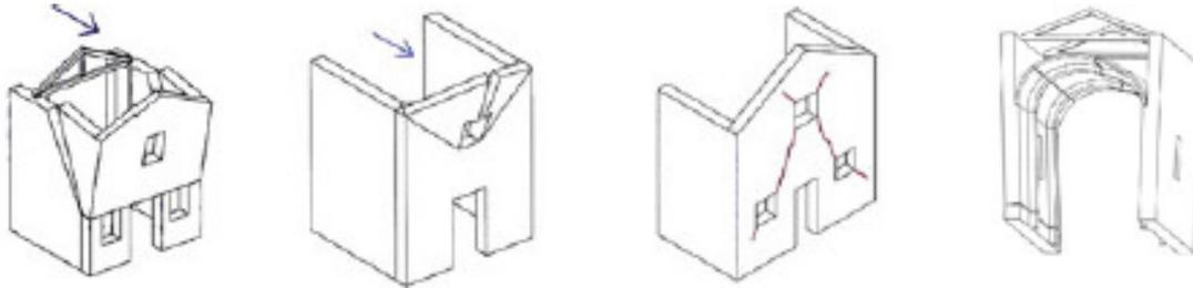
**Figure 15.** Some of the most common types of observed damage for the “Post-Byzantine Basilicas”
