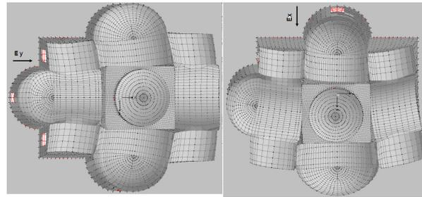
**Figure 14b.**  $E_y \delta_{\max} = 4.49\text{mm}$  at the top of the central dome.
