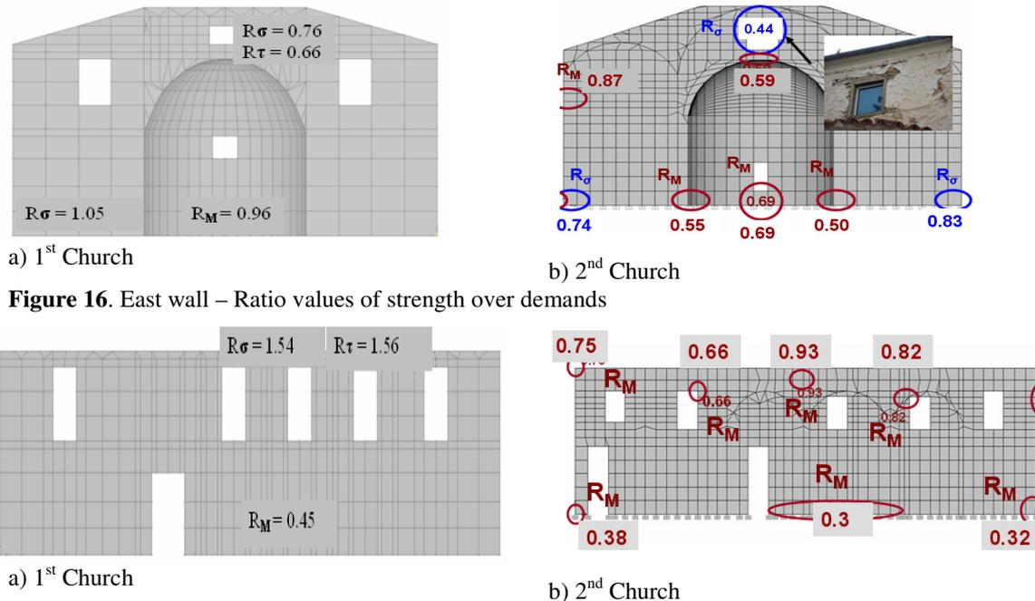
**Figure 17.** South wall – Ratio values of strength over demands
