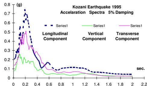
Figure 1b. Hor. acceleration response spectral curves of the main event ground motion recorded at the city of Kozani.
