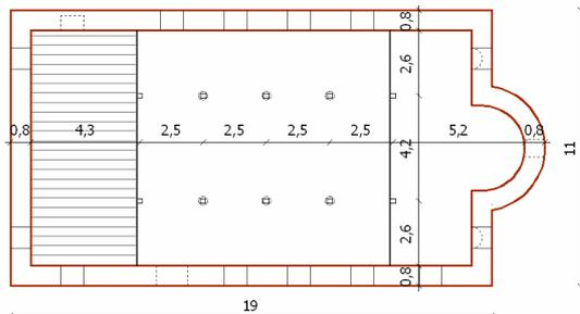
Figure 3a. 1<sup>st</sup> Post-Byzantine “Basilica” – plan
