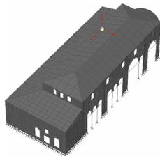
Figure 2a. The Basilica structural system with the interior colonnade of the central nave
