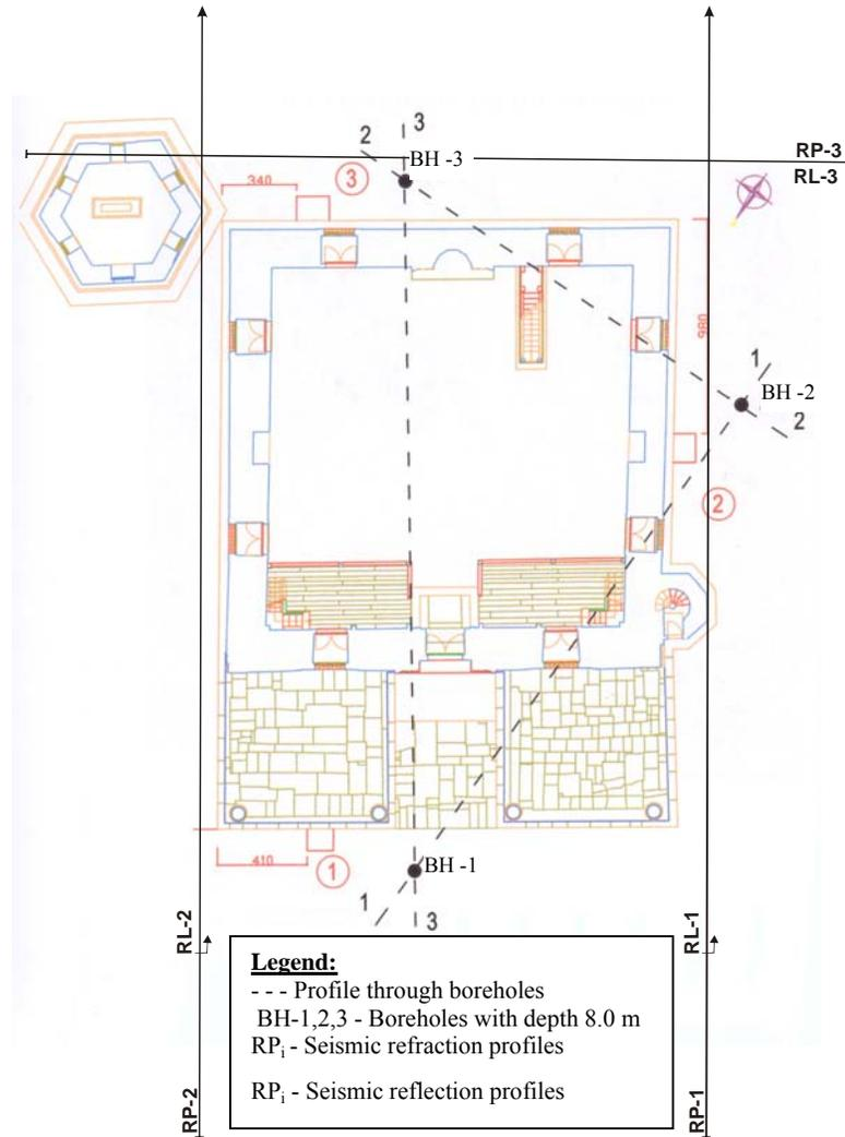
**Figure 3.** Site plan of performed geophysical and geotechnical investigation
