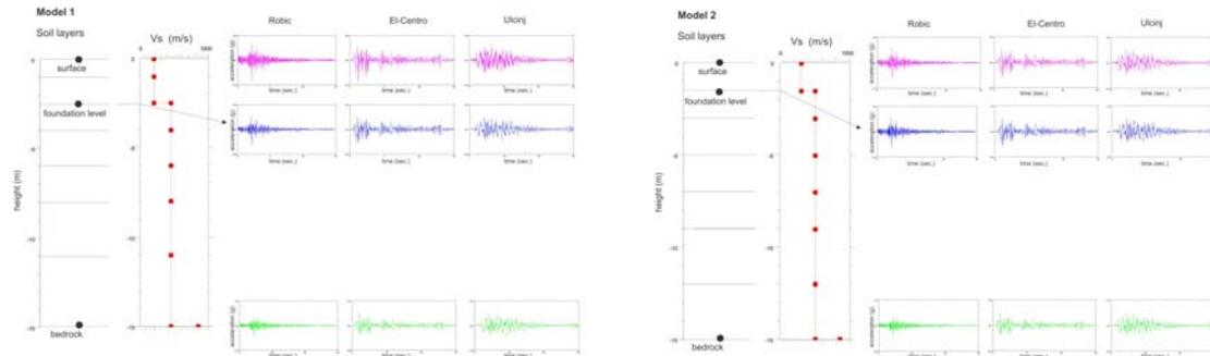
**Figure 9.** Seismic response of Model 1 (left) and Model 2 (right)-Time histories of acceleration for selected earthquake input
