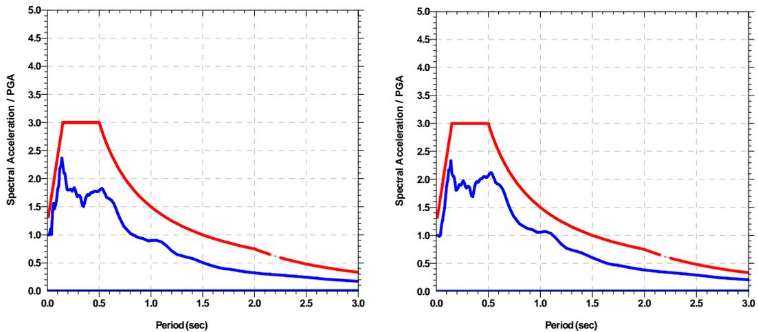
**Figure 8.** Mean normalized response spectrum for Model 1 (left) and Model 2 (right) and normalized spectrum in accordance with EC8 – ground type B, for 5% damping
