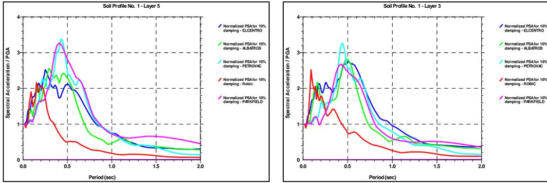
**Figure 5.** Mean normalized response spectrum for Model 1 (left) and Model 2 (right) for 10% damping
