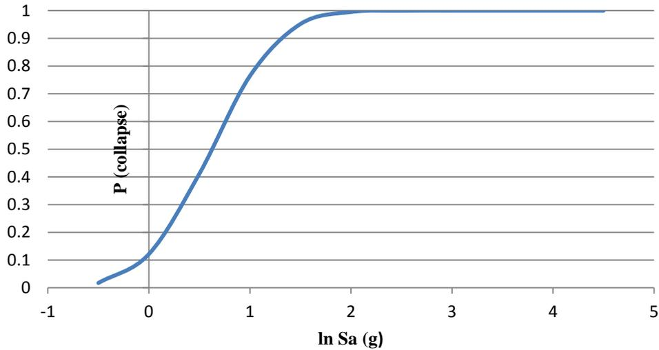
**Figure 8.1** Collapse fragility curve, Case 1
