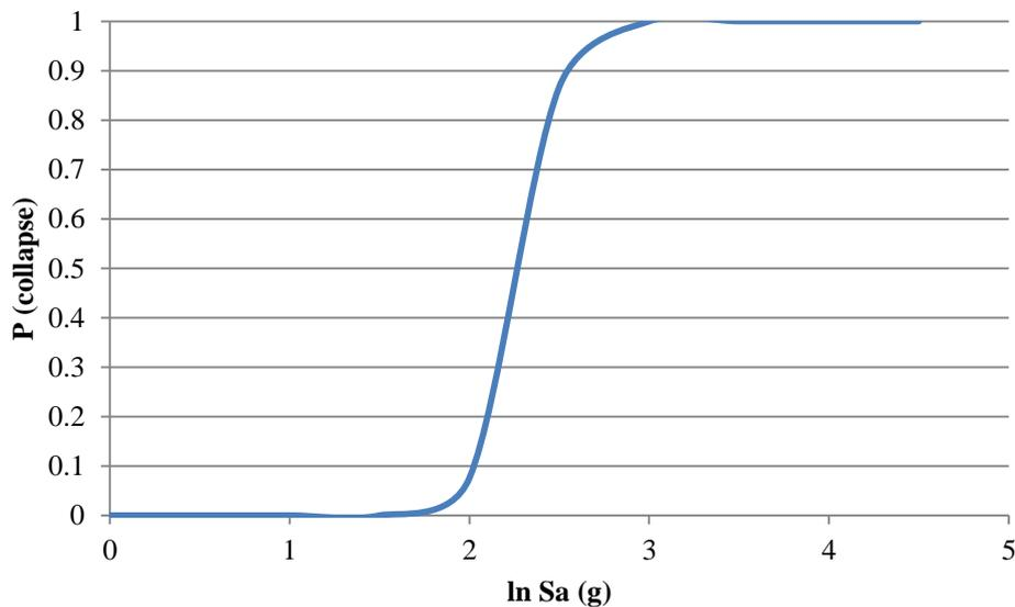
**Figure 8.2** Collapse fragility curve, Case 2
