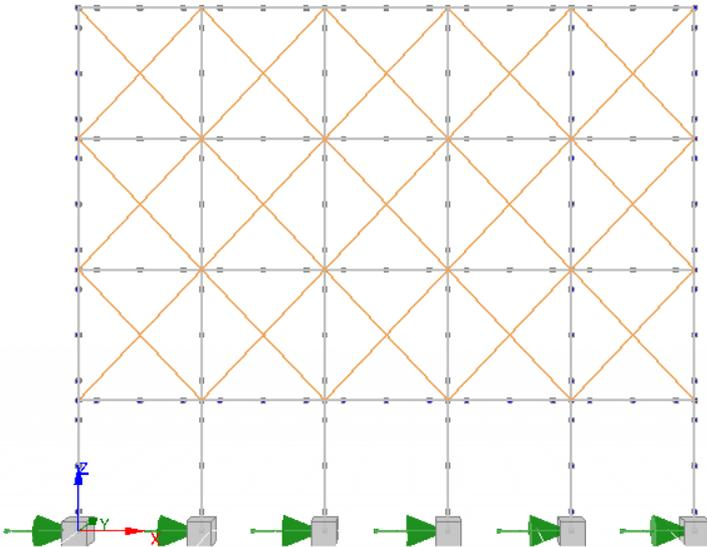
Figure 3.1 Analytical model with base excitation
