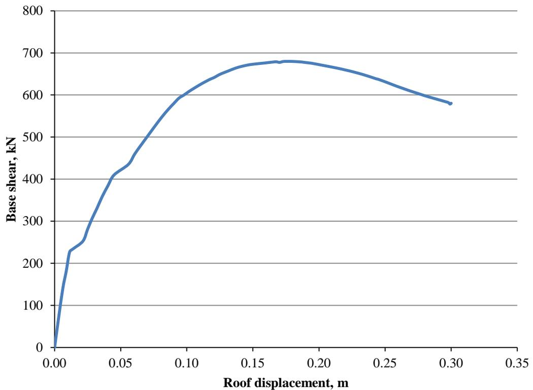
Figure 6.2 Pushover curve for example building (case 1)
