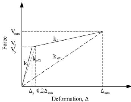
**Figure 3.** Design envelope curve for bilinear isolators
