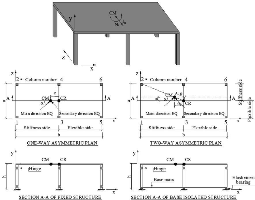
Figure 1. Structural models for investigation
