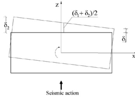
**Figure 2** Graphic of torsional irregularity in GB50011-2001 Code
