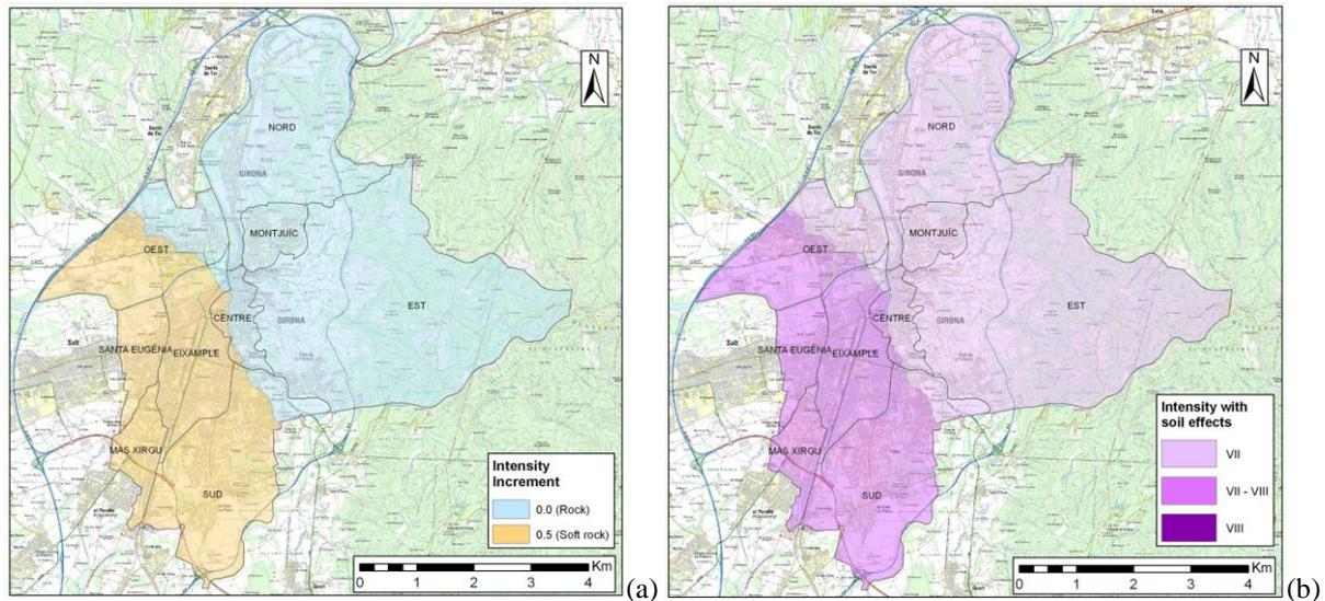
**Figure 3.1.** (a) Girona city microzonation map based on soil coefficient C; (b) Local hazard map for the city of Girona including the soil effects. (Vendrell, 2011).
