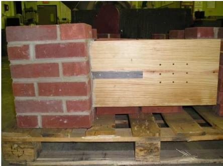
Figure 1. Test specimen of wall-diaphragm connection.
