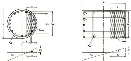
**Figure 3.** Behavior and parameters of the section analysis
