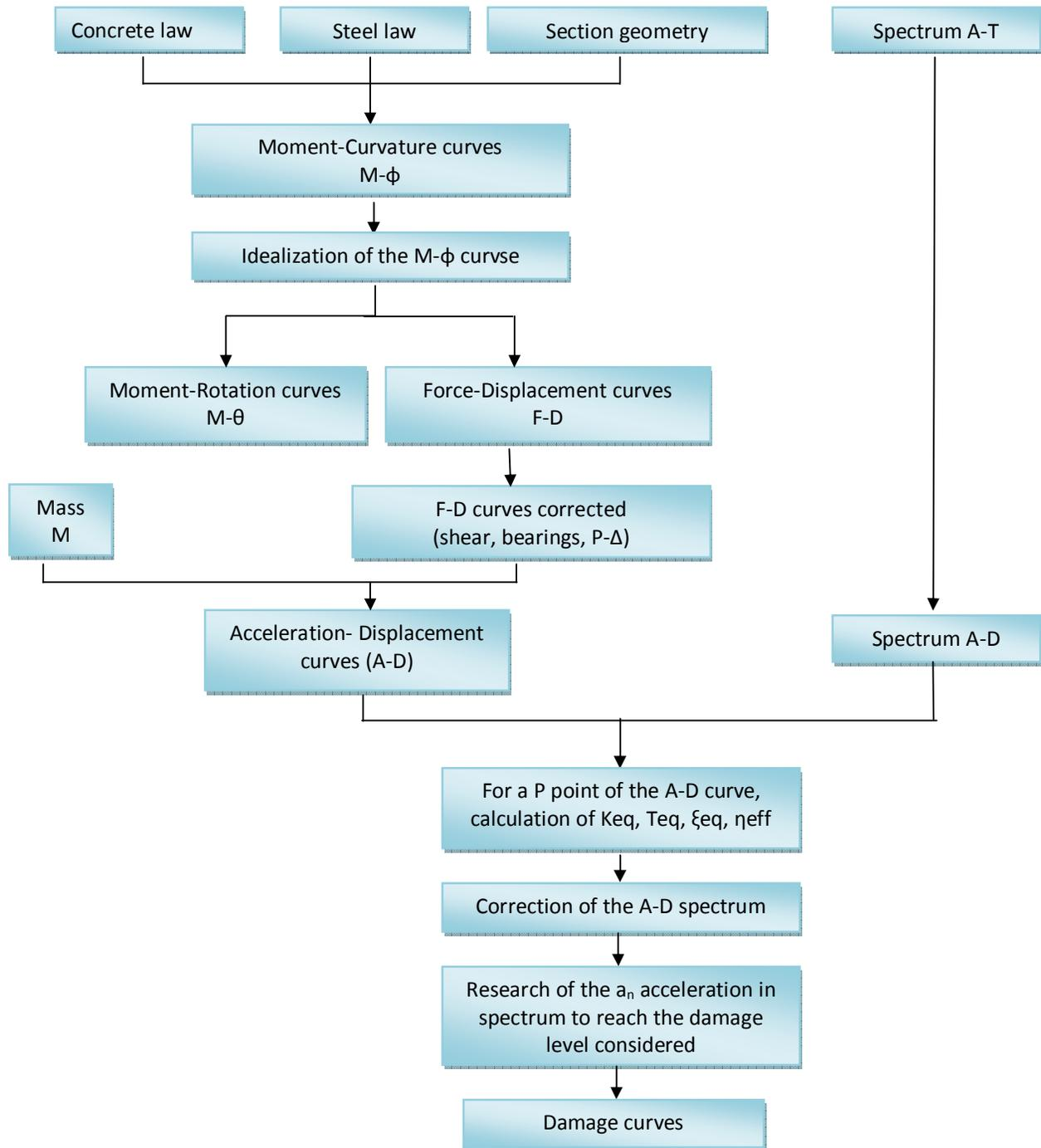
**Figure 1.** Pushover analysis developed in hand calculation
