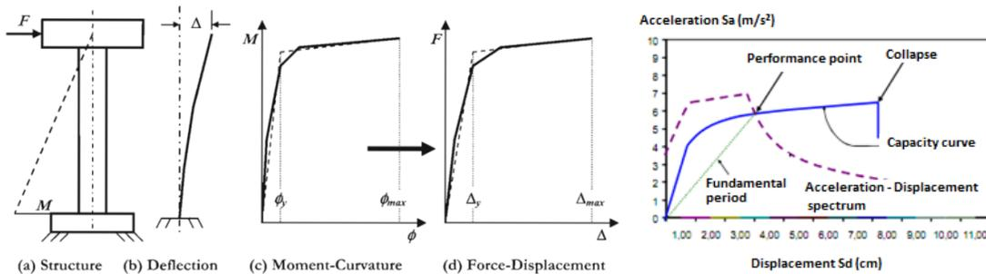
**Figure 2.** Principle of each step of the pushover analysis
