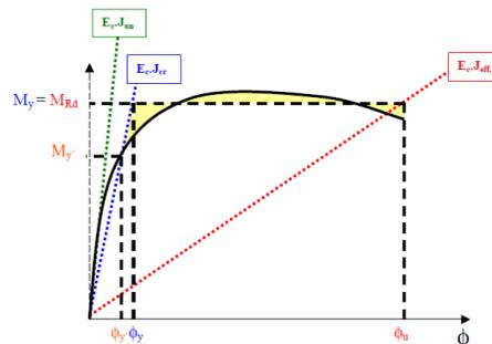
Figure 5. Idealization of the moment-curvature curve
