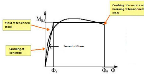
Figure 4. Moment-Curvature curve inflection points
