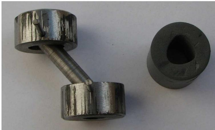
**Figure 1.** Prototype of the Elastomeric Polymer Bearing
