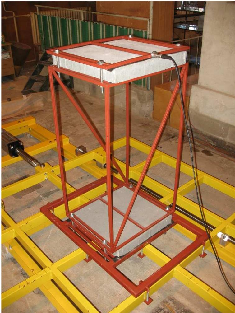
**Figure 3.** Non-isolated single-storey steel structure model mounted on the shaking table
