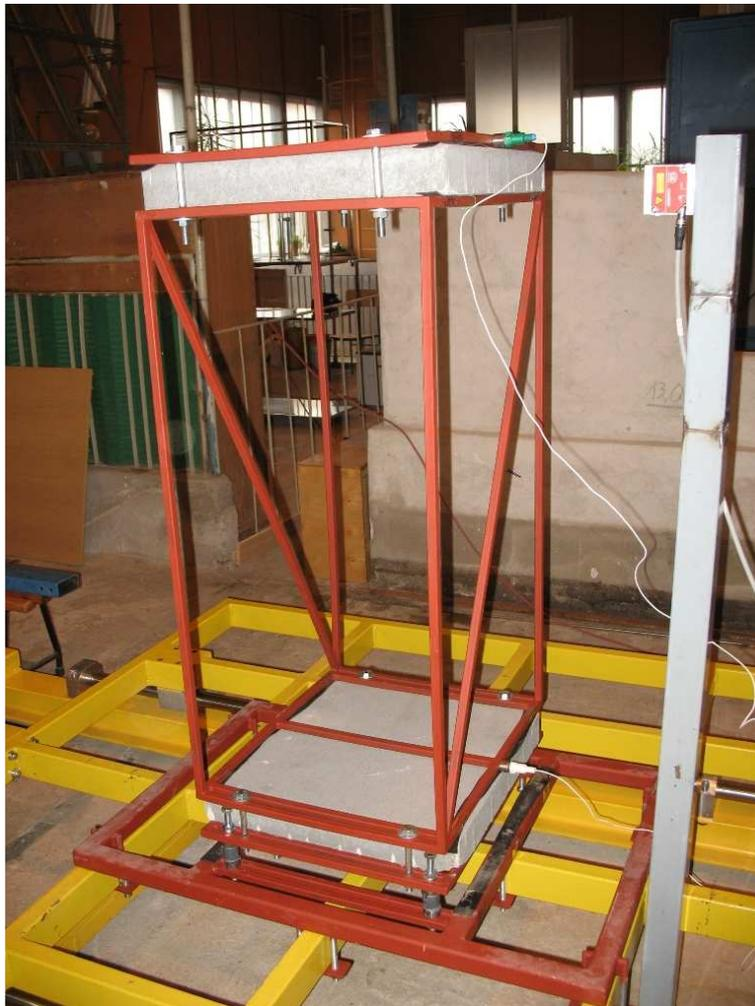
**Figure 4.** Base isolated single-storey model with two accelerometers and a laser displacement sensor
