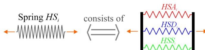
**Figure 3.5** Each horizontal spring is composed of 3 components to account for aggregate interlock (HSA), dowel (HSD) and shear/horizontal reinforcement (HSS) mechanisms
