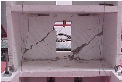
Figure 4.4 Shear failure in the first story
