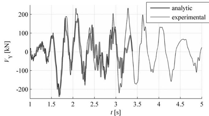
Figure 4.5 Base shear response in the direction of the web in the 6<sup>th</sup> run
