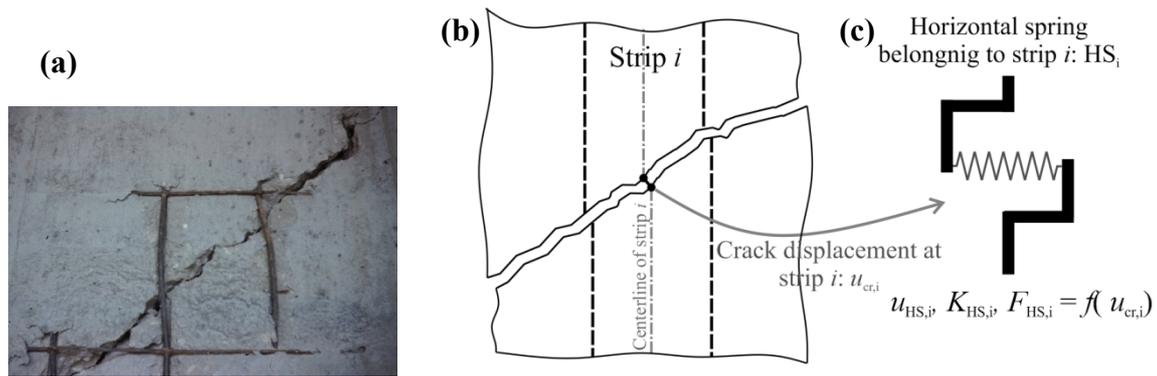
**Figure 3.3** Modeling of shear transfer mechanisms according to the proposed model: Each horizontal spring (c) represents the shear transfer mechanisms across cracks (a) for the assigned strip (b)
