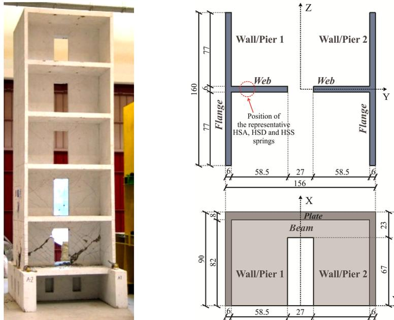
**Figure 2.1** The wall designed according to the Slovenian practice and tested on the shaking table at LNEC in Lisbon (Fischinger et al., 2006)
