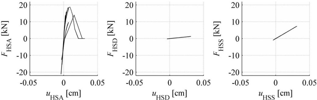
**Figure 4.3** Response of the shear springs accounting for different shear mechanisms in the 5<sup>th</sup> run
