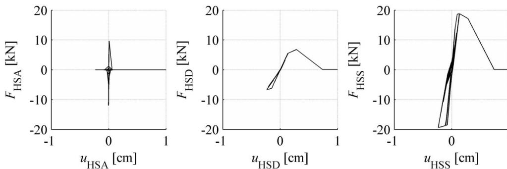
Figure 4.6 Response of the shear springs accounting for different shear mechanisms in the 6<sup>th</sup> run
