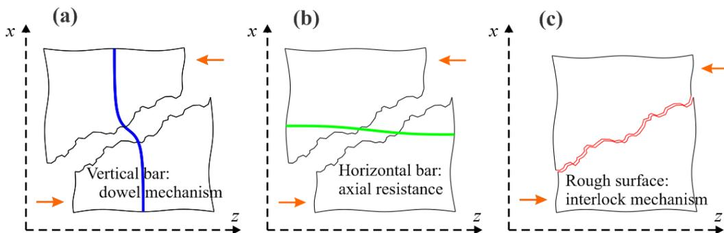
**Figure 3.4** Mechanisms of shear force transfer over the cracks: (a) dowel effect of vertical reinforcement; (b) axial resistance of horizontal/shear reinforcement and (c) interlock of aggregate in the crack
