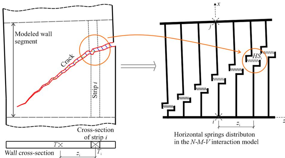
**Figure 3.2** Scheme of the upgraded MVLEM having multiple horizontal springs
