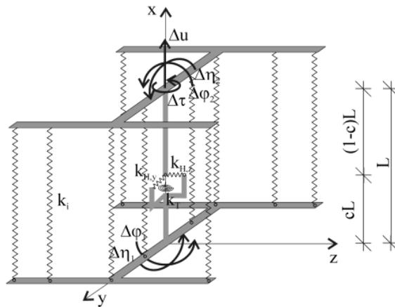
**Figure 3.1** 3D multiple-vertical-line-element (MVLEM)
