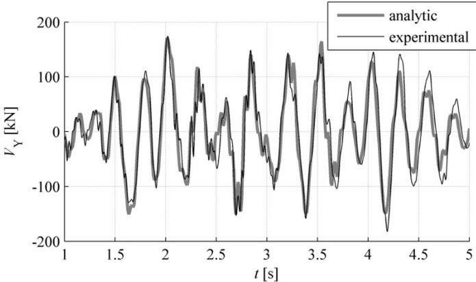
**Figure 4.2** Base shear response in the direction of the web during the 5<sup>th</sup> run
