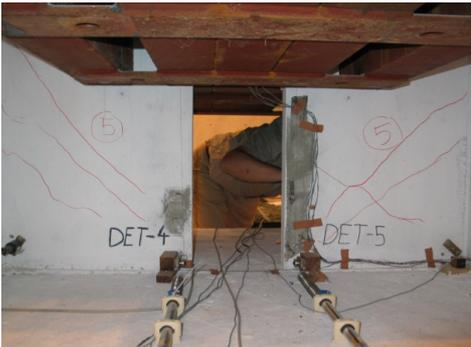
**Figure 4.1** Crack pattern in the web of the first story after the 5<sup>th</sup> run
