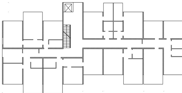
**Figure 1.1** Typical multi-story apartment building with structural walls
