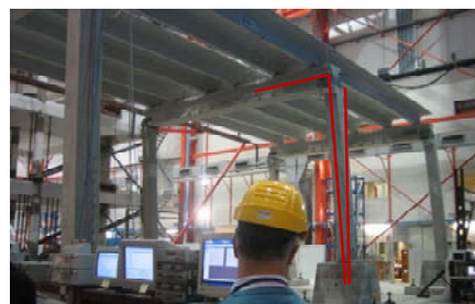
Figure 1.1. Large deformations (8% drift) of the columns in precast industrial building tested at ELSA in Ispra within the PRECAST project (Toniolo, 2007)
