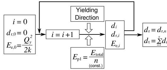
**Figure 4.** Procedure to compute the residual displacement under the hypothesis of constant energy input
