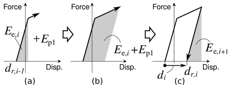
**Figure 3.** Assumed behavior during a single plastic deformation
