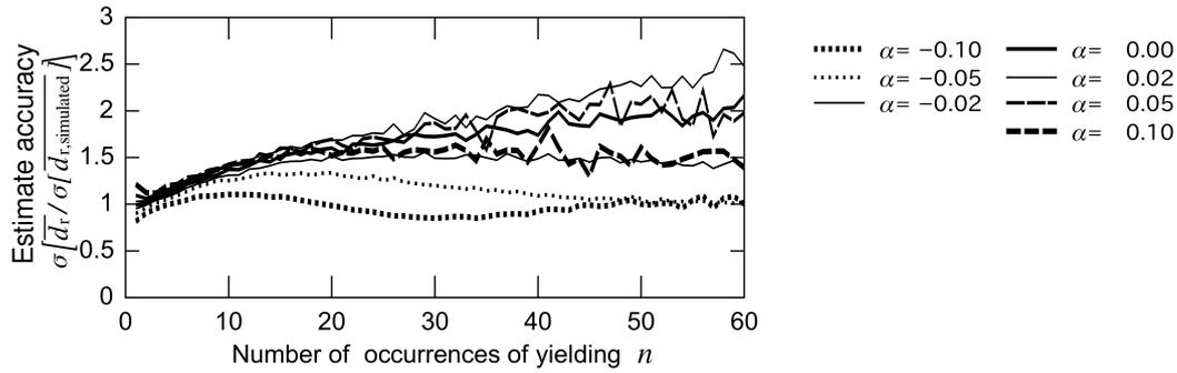
**Figure 7.** Accuracy of estimation by Monte Carlo simulation in case of kinematic hardening model
