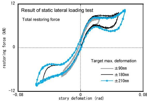
**Figure 2.5.** Relation between the whole restoring force and the relative story displacement
