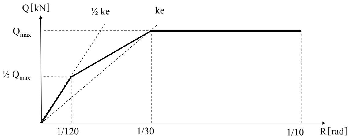
**Figure 3.4.** Restoring force characteristics of structural element
