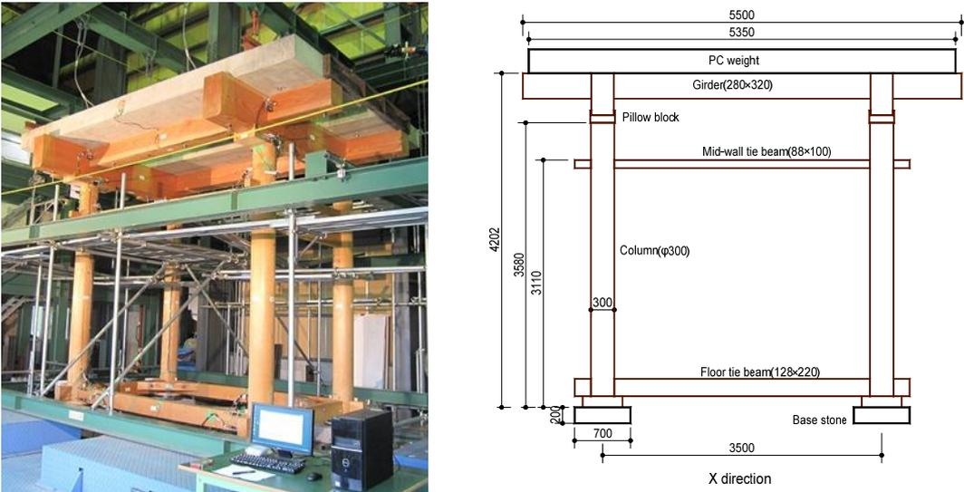
Figure 2.1. Overview and elevation plan of specimen
