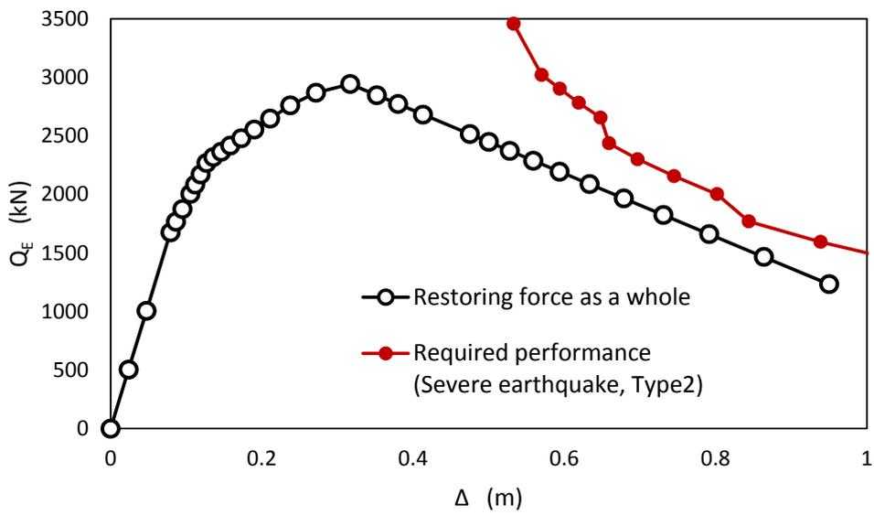
**Figure 3.6.** Seismic performance of X direction for Amida-do
