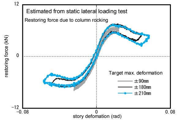
**Figure 2.6.** Restoring force due to column rocking
