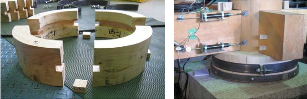
Figure 2.2. Reinforcement members and Situation of reinforced column bottom
