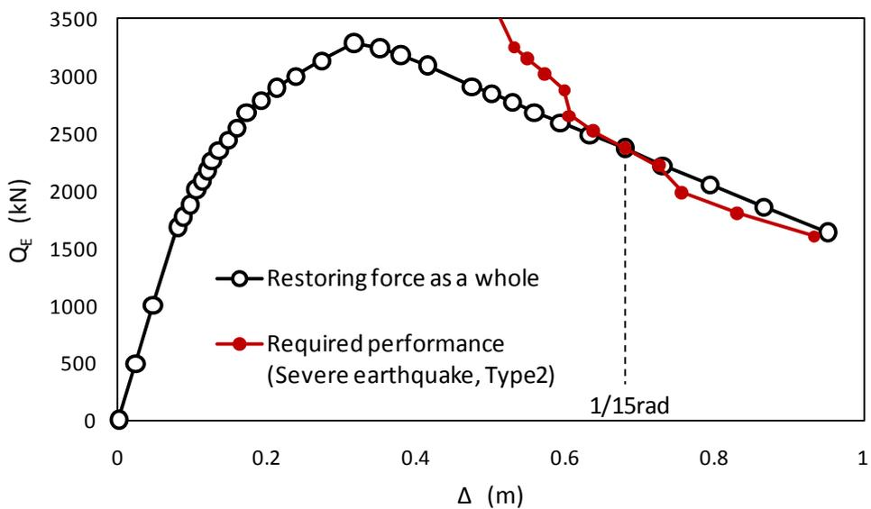
**Figure 3.7.** Seismic performance of X direction after reinforcement
