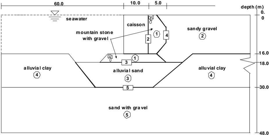
**Figure 3.** Typical Cross-section of the Finite Element Model
