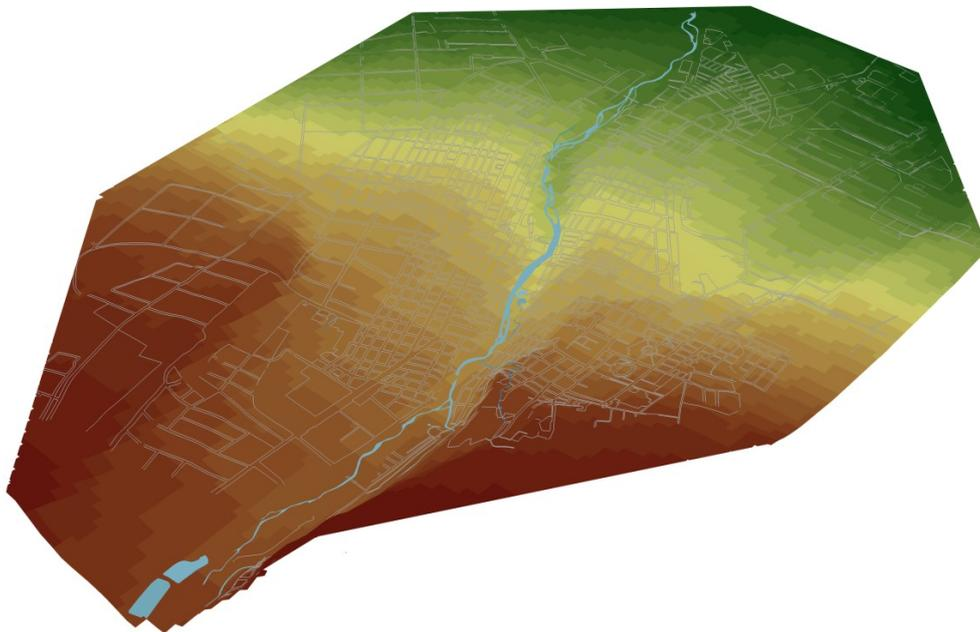
**Figure 4.** Digital elevation model of the territory of Vladikavkaz city (absolute height varies from 630 (green) to 750 meters (brown))
