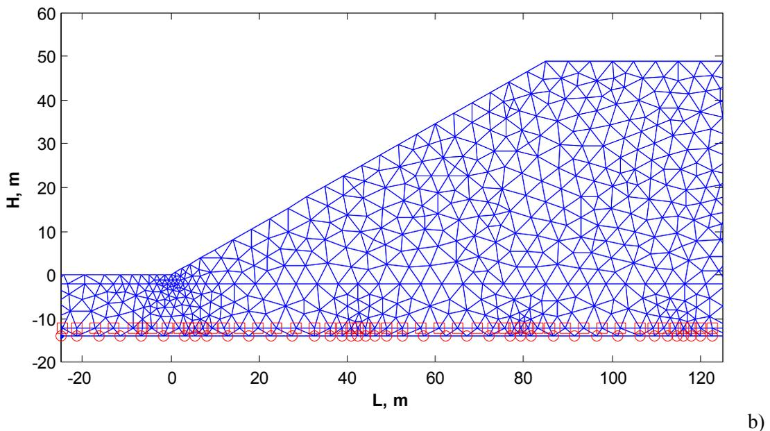
**Figure 3.** Amplification of vibrations along slope (1 – calculated; 2 -- instrumental) and calculational model of slope
