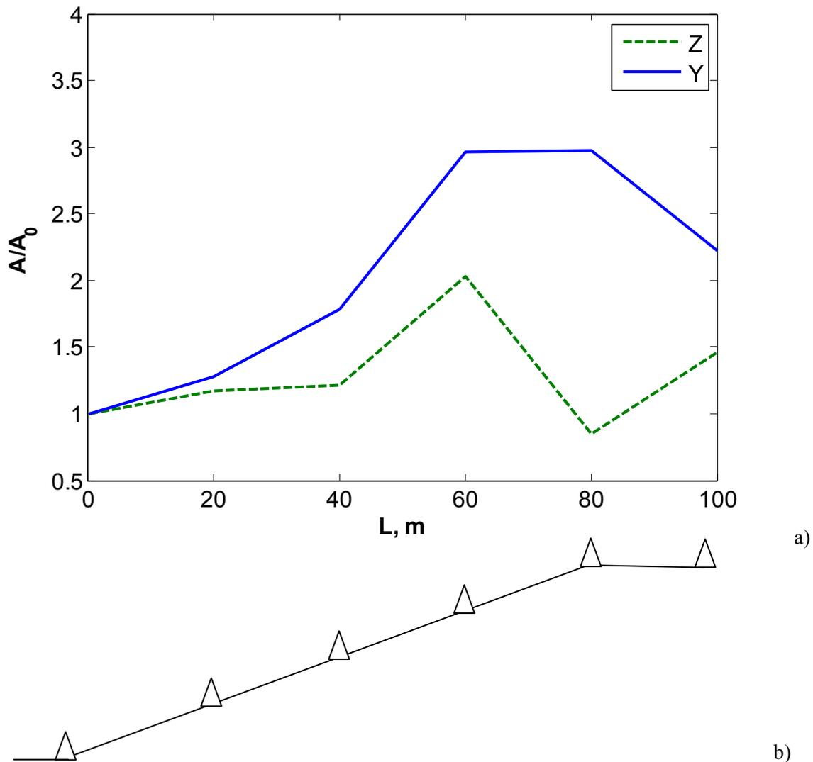
**Figure 2.** Amplification of microseisms amplitudes  $A/A_0$  (a) along slope (b)
