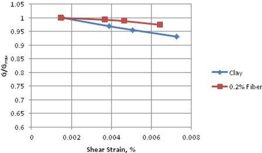
**Figure 2.** Shear modulus degradation graph of clay and fiber reinforced clay
