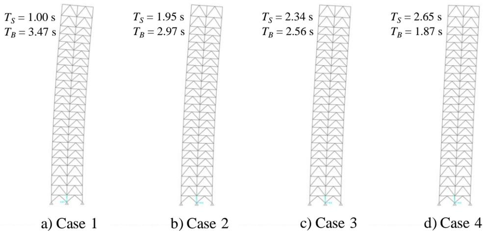
**Figure 3.** Fundamental mode of vibration for all versions of bracing sub-system
