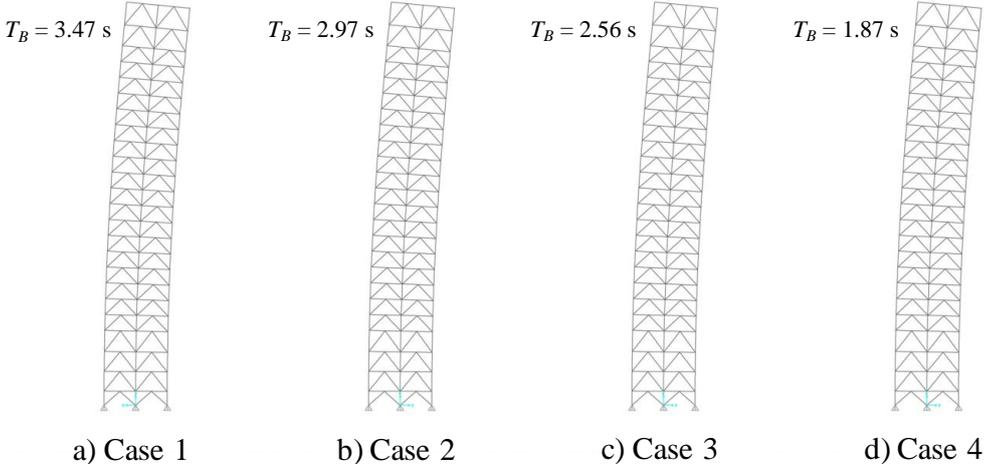
**Figure 5.** Fundamental mode of vibration due to global flexural drift mode for all versions of bracing system
