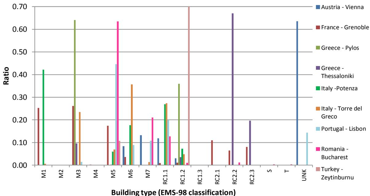
**Figure 1:** TBA Distributions in EMS-98 Classification of building types.
