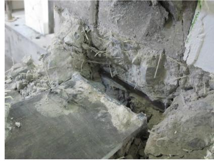
**Photo 3.2.** Fracture of steel beam of Specimen CWPS (Observation after test)
