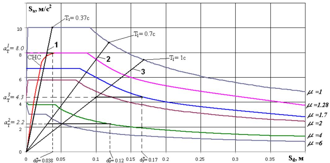
**Figure 3.** Examples to determine the nonlinear displacements  $d$  of three buildings (1, 2 and 3) with different values of period  $T_1$ , yield limit and ductility coefficient for soils of the 2-nd category using seismic characteristics at earthquake intensity of 9 points on scale [18]
