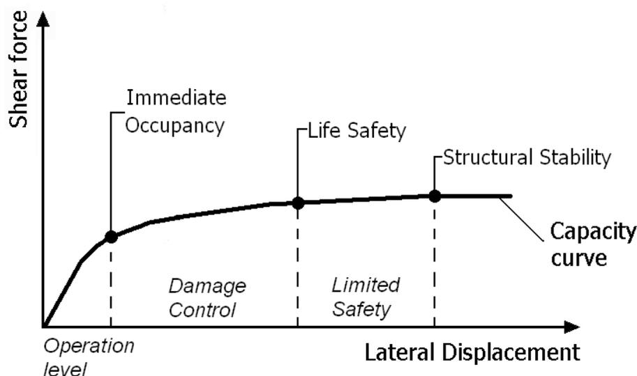
**Figure 1.** Relations between summarized forces and displacements for different operation levels corresponding to base shear-displacement capacity curve
