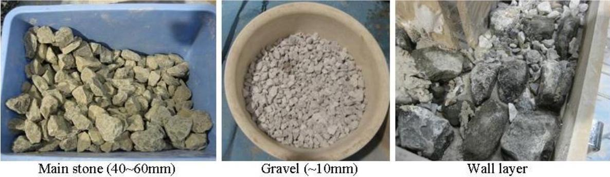
**Figure 6.** Detail of stone used for construction.
