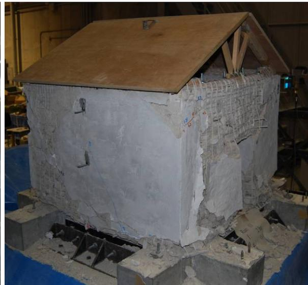
**Figure 15.** Retrofitted model after Run 51
