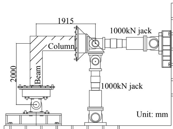
**Figure 3.** Loading Apparatus
