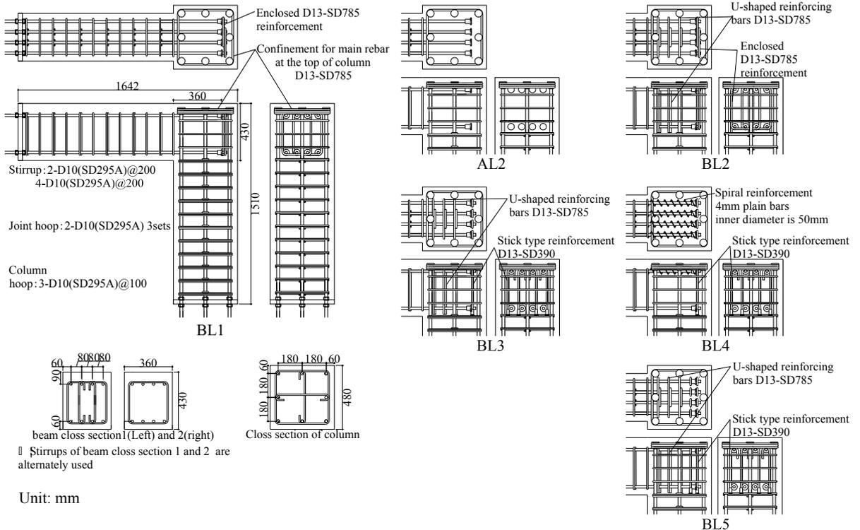
**Figure 1.** Reinforcement of Specimens
