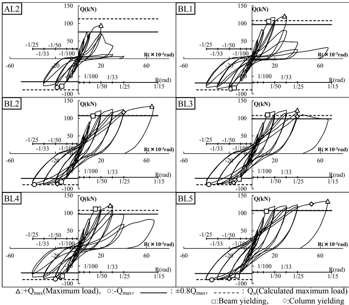
Figure 4. Story Shear  $Q$  vs. Story Drift  $R$  Relationship
