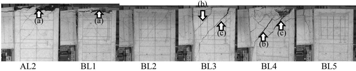
Photo 1. Damage View at Amplitude Peak, AL2:  $R=+ 1/25\text{rad}$ , Others:  $R=+ 1/15\text{rad}$
