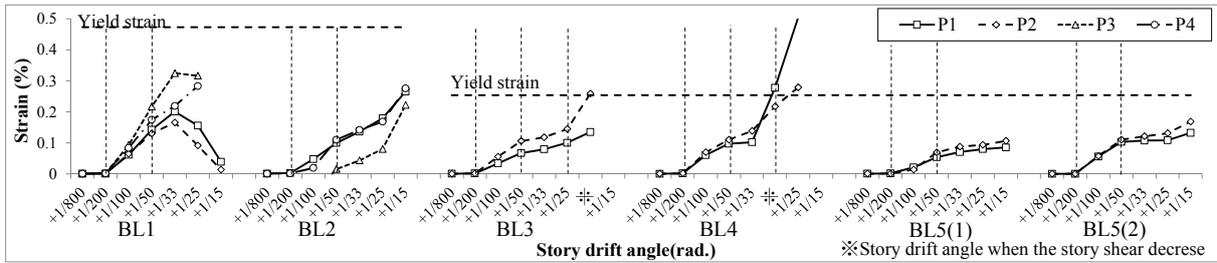
Figure 6. Change of Strain in Enclosed Reinforcement (BL1, 2) and Stick Type Reinforcement (BL3, 4, 5)
