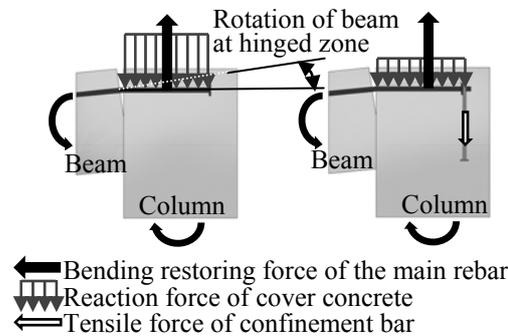
**Figure 2.** Resisting Mechanism of Beam Main Rebar Anchored in Joint
