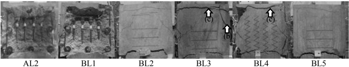
Photo 3. Damage View of Column Top after Loading
