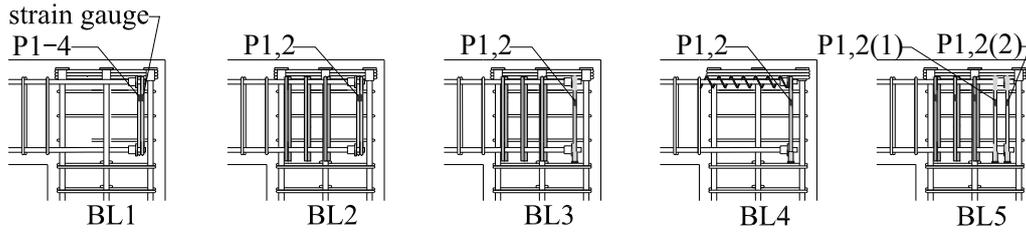
Figure 5. Location of Strain Gauges of Reinforcement
