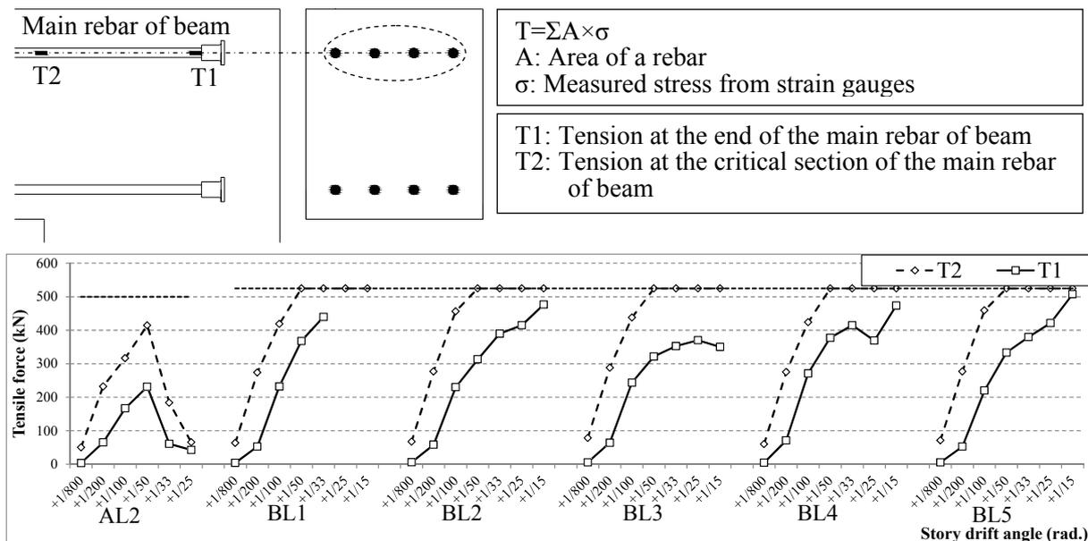
Figure 7. Change of Bearing Force T1 and Tensile Force T2 of Beam Main Rebar
