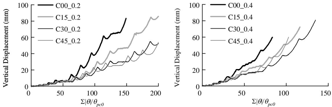
**Figure 7.** Vertical Displacement-Cumulative Deformation Relationships
