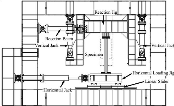
Figure 3. Elevation of the Loading System
