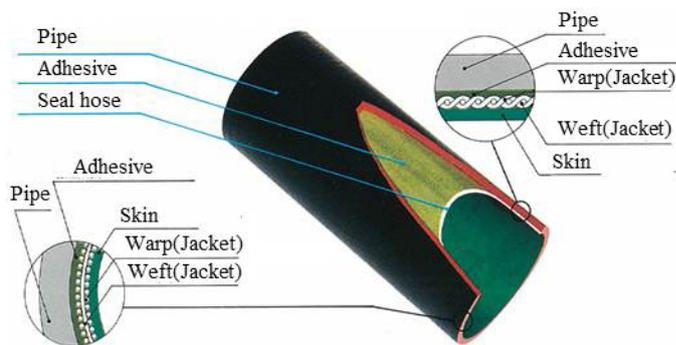
**Figure 2.1** Cross section of a hose-lined pipe
