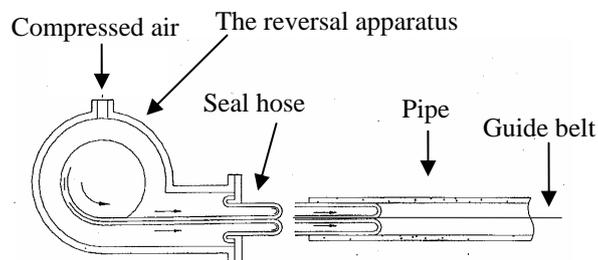
**Figure 2.3** Schematic diagram of hose-lining apparatus
