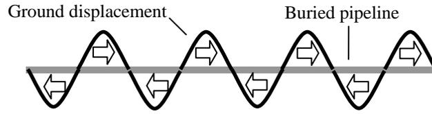
**Figure 7.1** Ground displacement acting on buried pipeline
