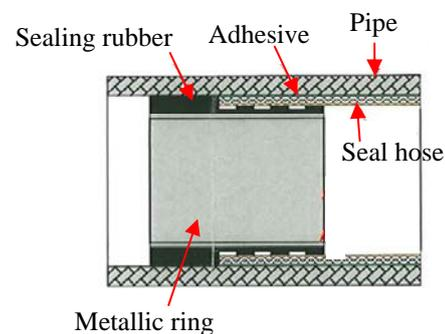
**Figure 2.2** Schematic diagram of the end part
