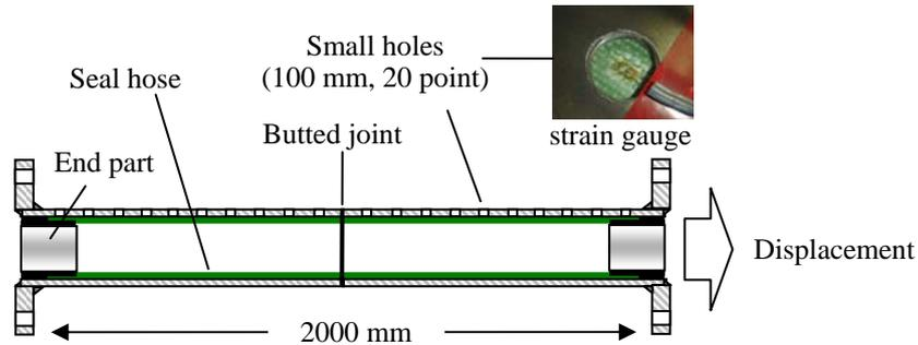
**Figure 5.1** Test Specimen
