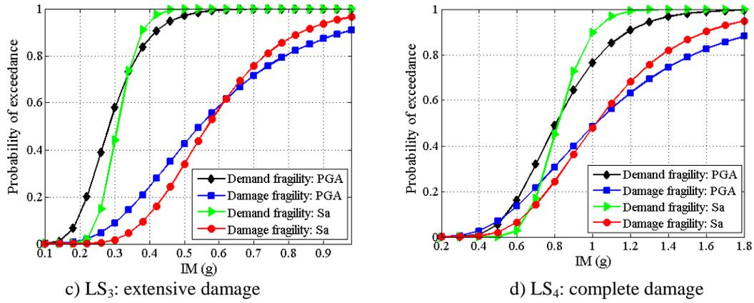
**Figure 2.** Seismic demand and damage fragility curves
