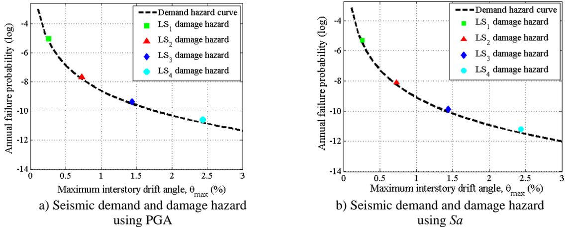
**Figure 3.** Seismic demand and damage hazard curves
