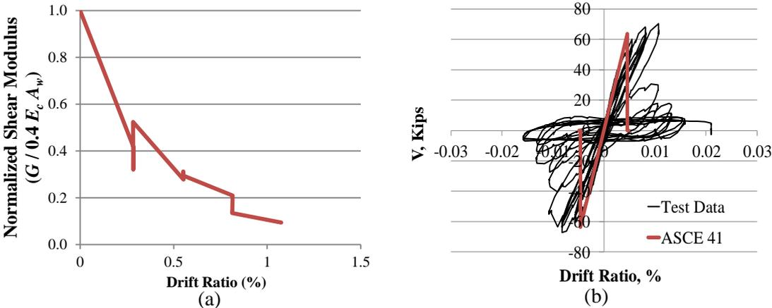
Figure 1. Normalized shear modulus and hysteretic response of column 3.
