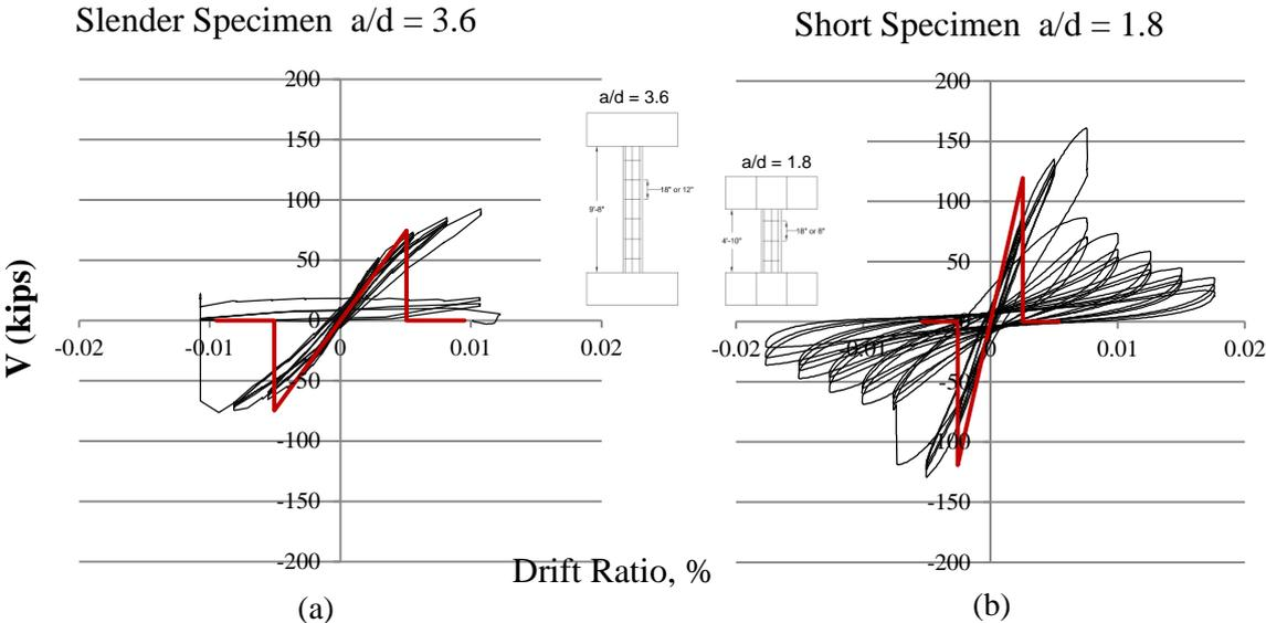
**Figure 2.** Hysteretic response for column specimens with different shear span-to-depth ratio. Both specimens had a longitudinal reinforcement ratio of 2.5%, #3 hoops with 90 deg. ties at 18 in. and an axial load of 500 kips.
