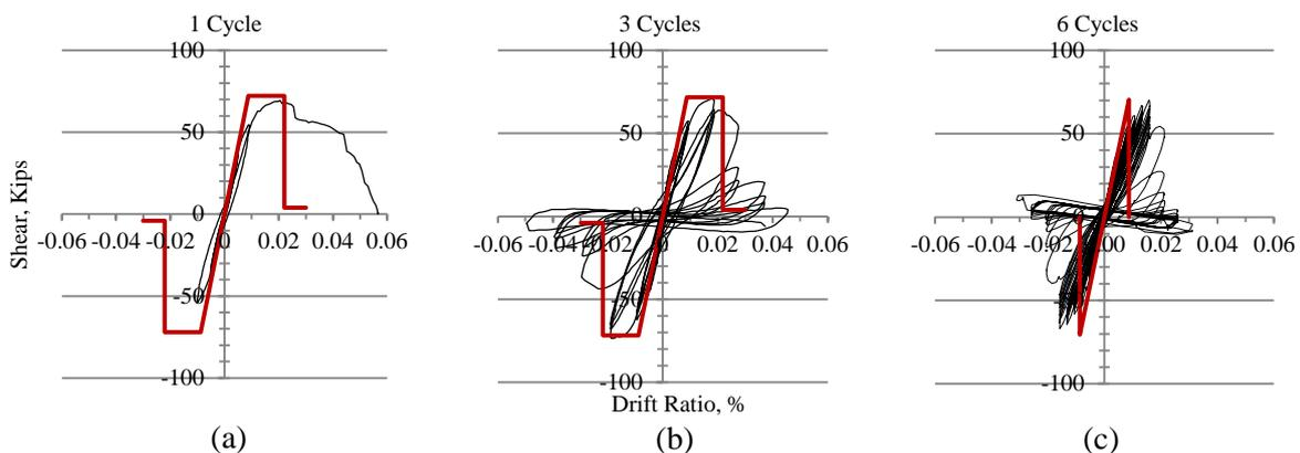
**Figure 5.** Hysteretic response of three columns subjected to different number of cycles per drift ratio. All columns had a longitudinal reinforcement ratio of 2.5%, diamond and rectangular ties spaced at 12 in., and an axial load of 150 Kips.
