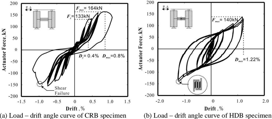
(a) Load – drift angle curve of CRB specimen (b) Load – drift angle curve of HDB specimen
