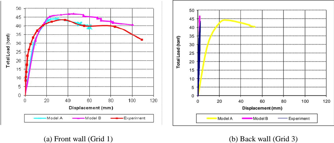
**Figure 5.1.** Comparison of experimental and analysis results
