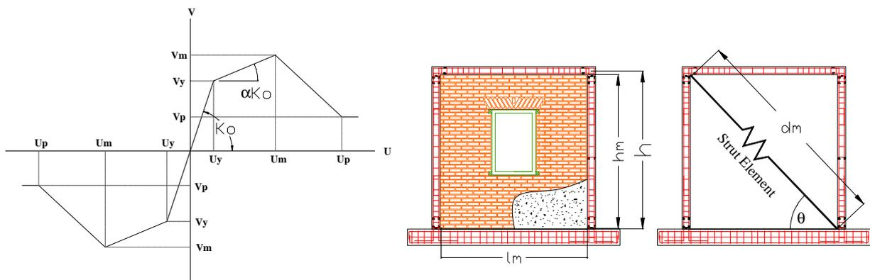
**Figure 2.1.** Masonry infill panel modelled as strut element
