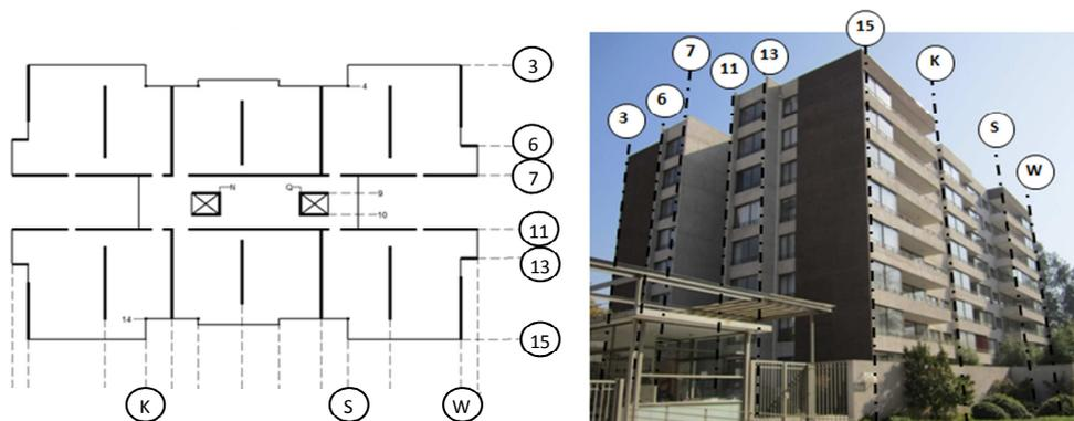
**Figure 2.** Typical floor plan and core elevation of a “fish-bone” Chilean residential building in Santiago
