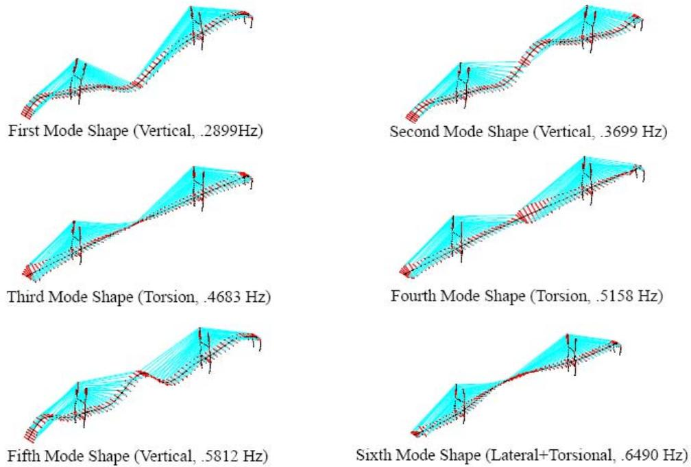
**Fig. 6.1** Modal characteristics of original FEM model [Dyke *et. al.* (2000)]
