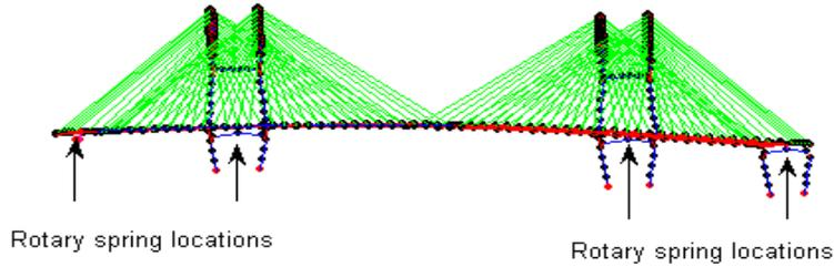
**Fig. 5.7** Finite element model with added rotary springs
