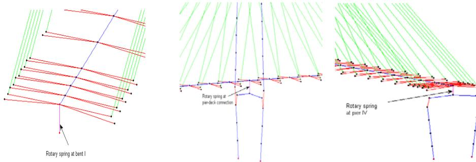
**Fig 5.8** Spring connection in close view
