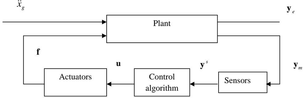
**Fig. 4.1** Block diagram representation of active control system
