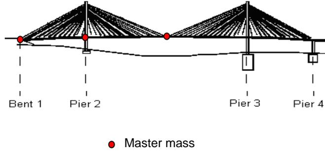
**Fig. 5.6** Locations of master masses in the finite element modal
