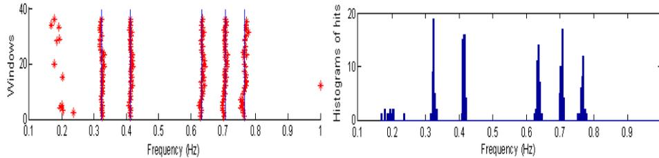
**Fig. 5.5** Details of modal identification by SSI
