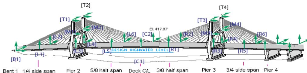
**Fig. 5.2** Locations of sensors in the bridge
