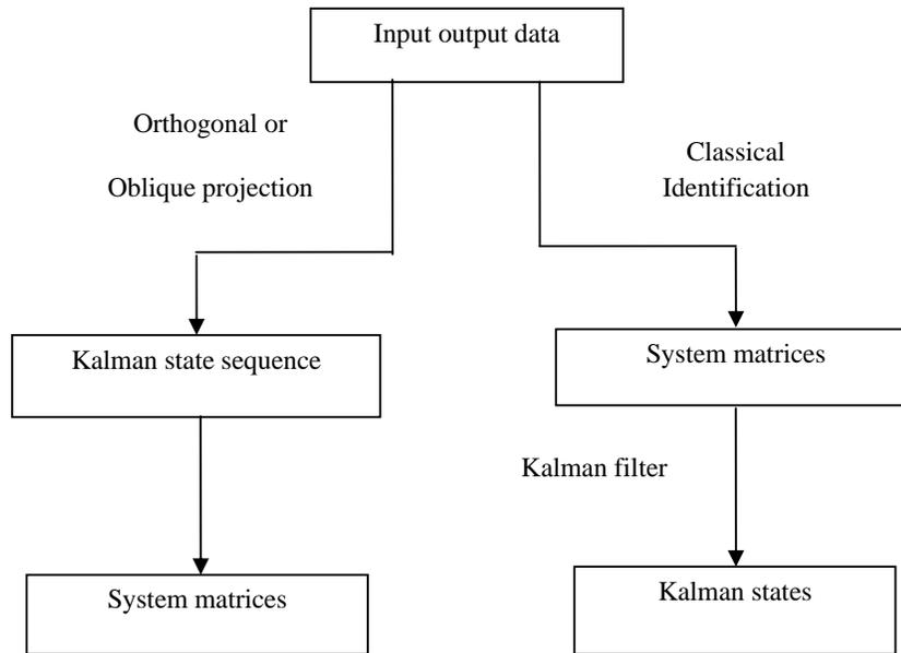
**Fig. 5.1** Comparison between subspace method and classical method
