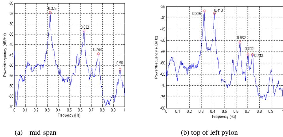
**Fig. 5.4** Power Spectral Density of signals for two key locations
