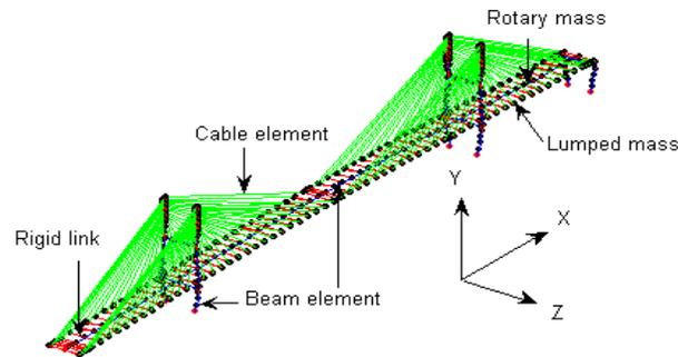
**Fig. 3.1** Finite element model
