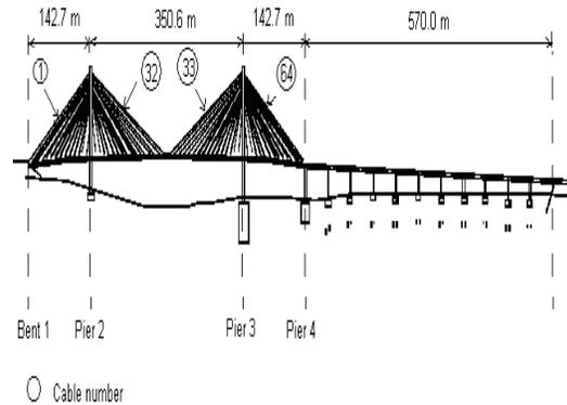
(b) Line diagram of bridge [Dyke *et. al.* (2003)]
