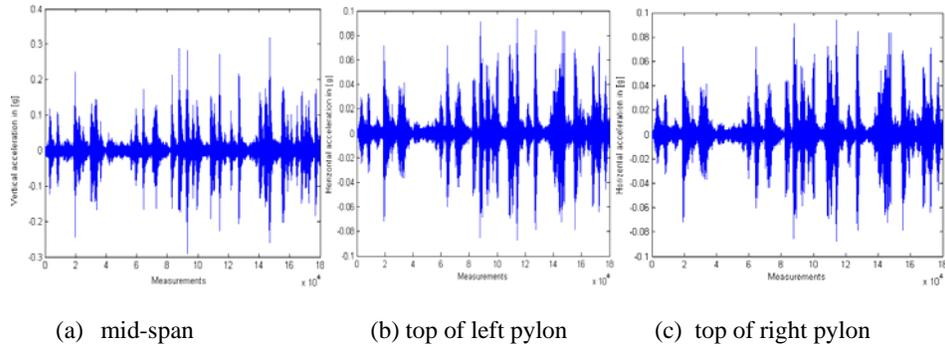
**Fig. 5.3** Sensor signals at three key locations
