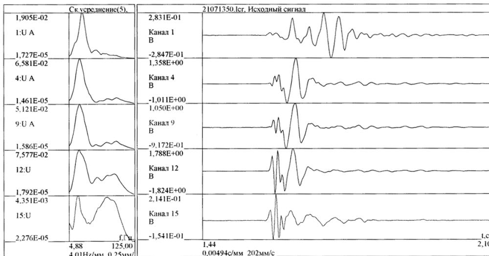
**Fig. 3.** Occurrence of a significant HF component in the near field of a powerful non-explosive pulsed source of GSK-6M
