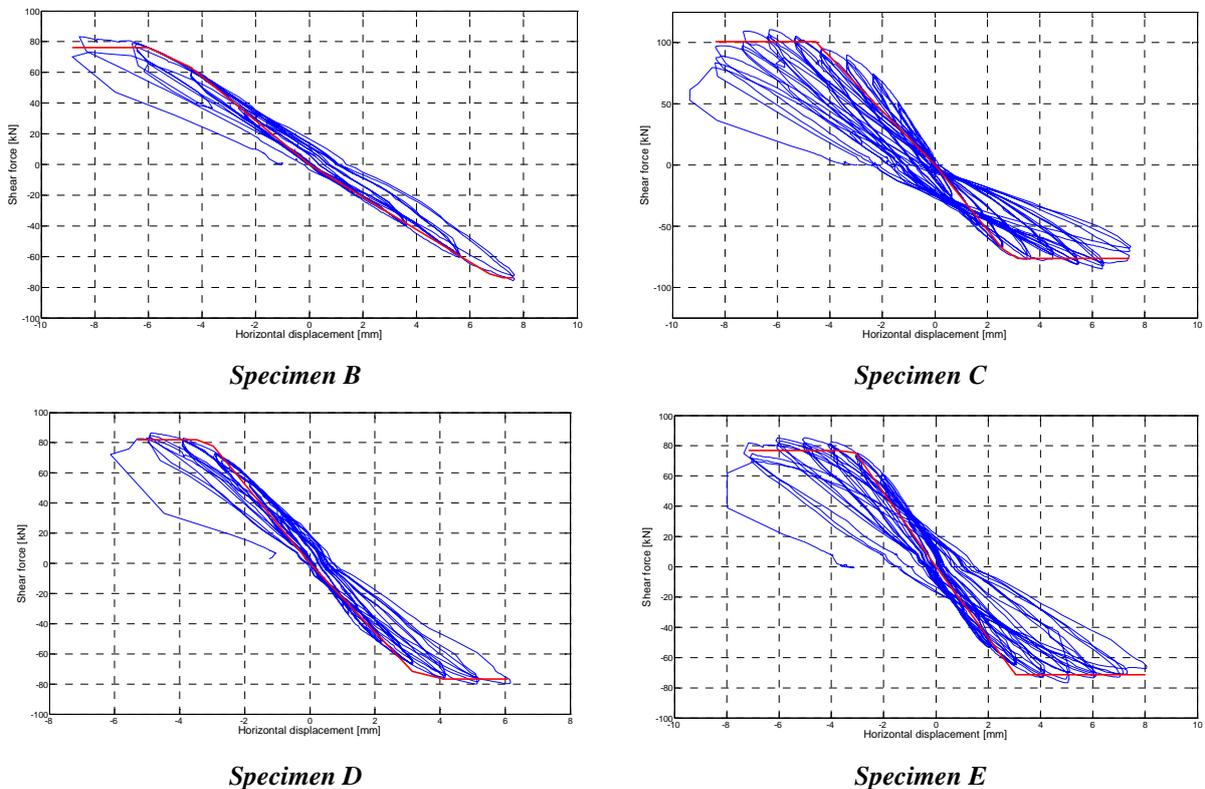
**Figure 4.4. Horizontal cyclic behaviour**
