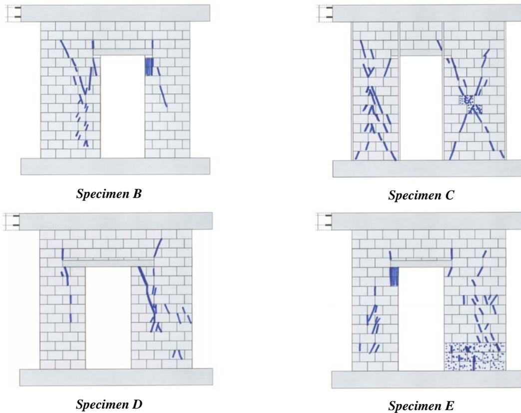
Figure 4.5. Crack patterns.
