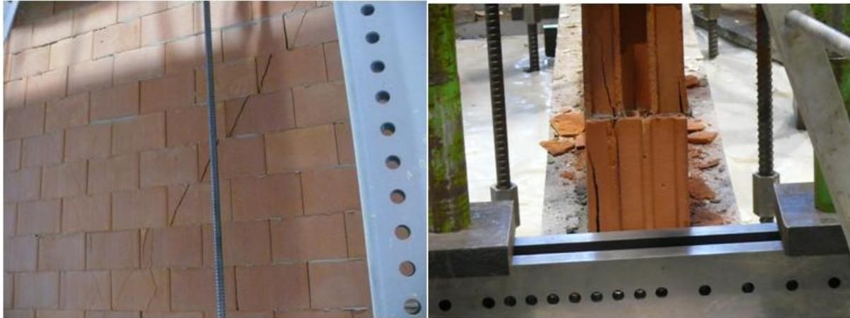
**Figure 4.3 (a) Diagonal cracking - (b) Crushing of the toe**
