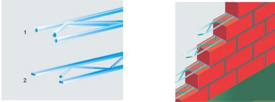
**Figure 3.3.** Horizontal reinforcement of specimen E.
