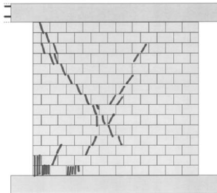
**Figure 4.2.** Final crack pattern of the full wall.
