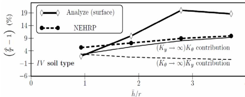
**Figure 9.** Variation of fundamental periods with  $\bar{h}/r$  ratios in surface foundations (soil type IV)
