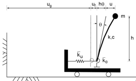
Figure 1. Experimental model of SSI system [Stewart J., P., et al 1998]
