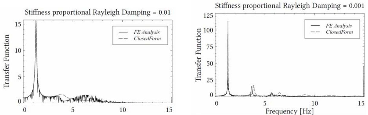
**Figure 5.** Transfer function of finite element and closed form solutions
