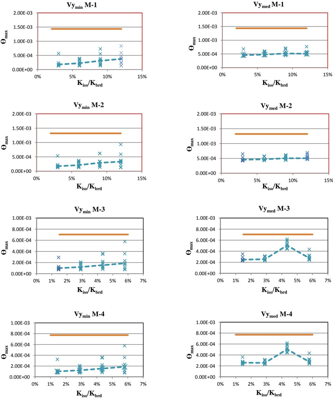
Figure 3. Drift demands in transverse direction in short piers (M-1 to M-4 models)
