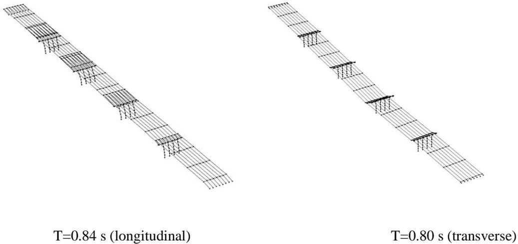
**Figure 2.** First two shape modes of the model M-1
