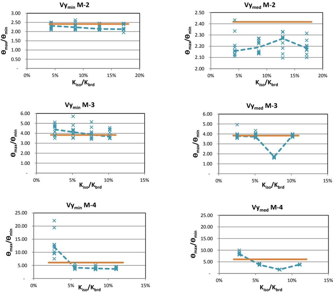
**Figure 4.** Ratios of the maximum to the minimum drift demands on piers in the transverse direction of the bridge models M-1 to M-4
