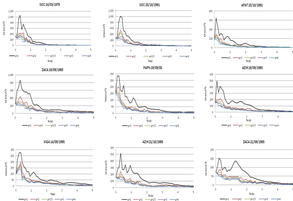
**Figure 1.** Elastic and inelastic response spectra of the selected seismic records
