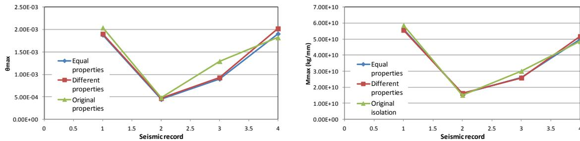
**Figure 8.** Drift and bending moment demands in piers for the seismic action in longitudinal direction
