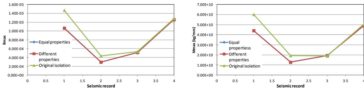
**Figure 7.** Drift and bending moment demands in piers for the seismic action in transverse direction
