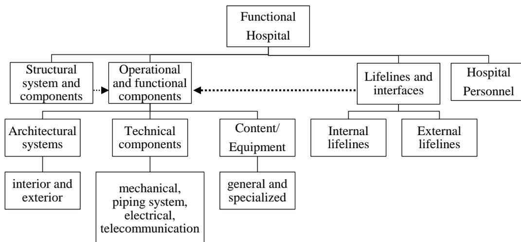
**Figure 3.1.** Functional components of a hospital
