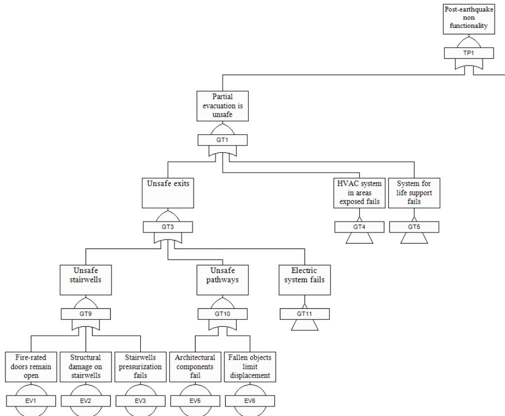
Figure 5.1. Fault tree for “unsafe partial evacuation”
