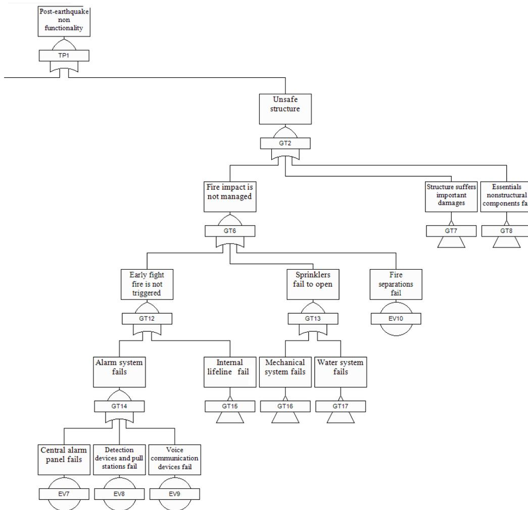
**Figure 5.2.** Fault tree for “unsafe structure”
