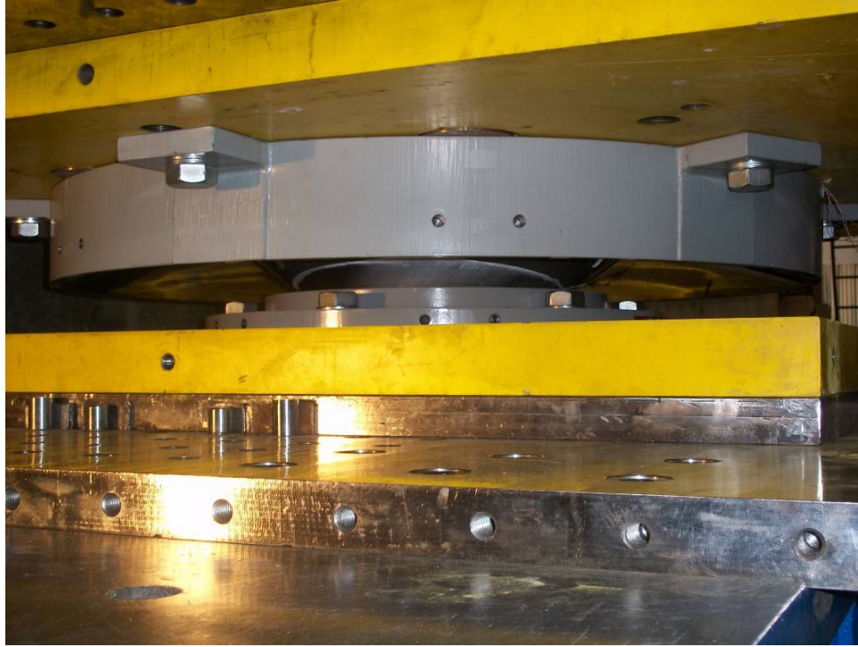
Figure 9. Test performed on the friction pendulum
