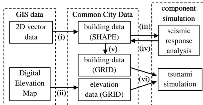
Figure B.1. Integration of simulations using Common City Data, in detail.
