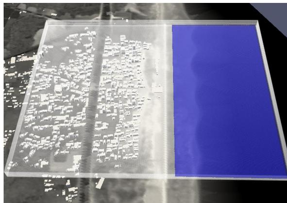
**Figure 3.5.** Analysis domain of tsunami simulation. Blue indicates the input tsunami wave.
