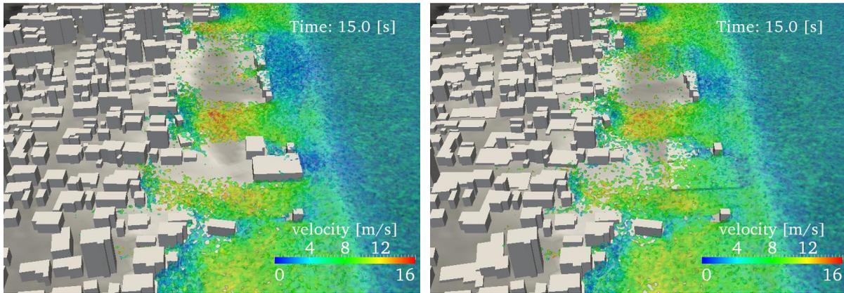
**Figure 3.7.** Close up view of results of tsunami simulation. Colors indicate fluid velocity. Left: tsunami simulation results without regarding, right: with regarding structural damage due to strong ground motion.
