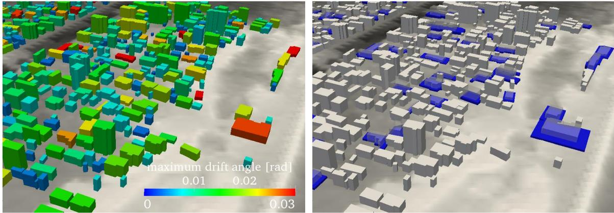
**Figure 3.4.** Modification of city model based on SRA results. Left: maximum drift angle of buildings. Right: modified city model, blue indicate collapsed shape of buildings, where transparent indicate the original shape.
