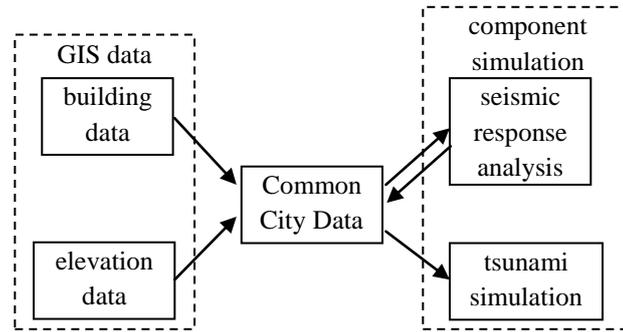
**Figure 2.1.** Integration of simulations using Common City Data
