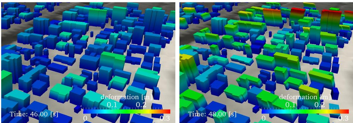
**Figure 3.3.** Close up view of seismic response analysis results. Colors indicate magnitude of deformation. Deformation is magnified by 20 times.
