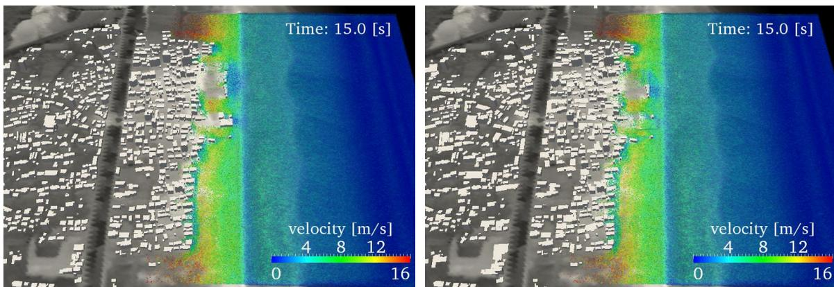
**Figure 3.6.** Overview of results of tsunami simulation. Colors indicate fluid velocity. Left: tsunami simulation results without regarding, right: with regarding structural damage due to strong ground motion.
