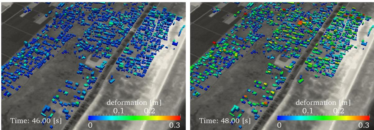
**Figure 3.2.** Overview of seismic response analysis results. Colors indicate magnitude of deformation.
