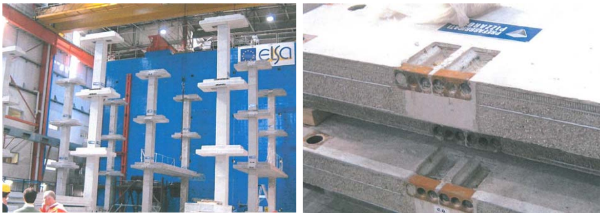
Figure 2. Whole columns with cross shaped corbel for the support of the shallow hollow core beam and detail of one beam edge. Note the rough surfaces for better interlock, the innovative mechanical connections placed in correspondence of the column and the hole for the dowel connection, in correspondence of the rib
