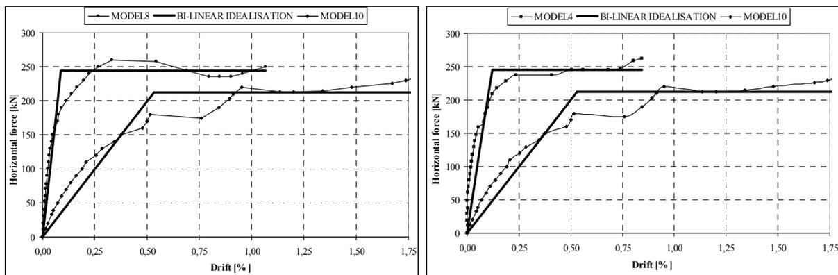
Figure 9 Idealisation of experimental hysteretic behaviour for MODEL8 and MODEL4
