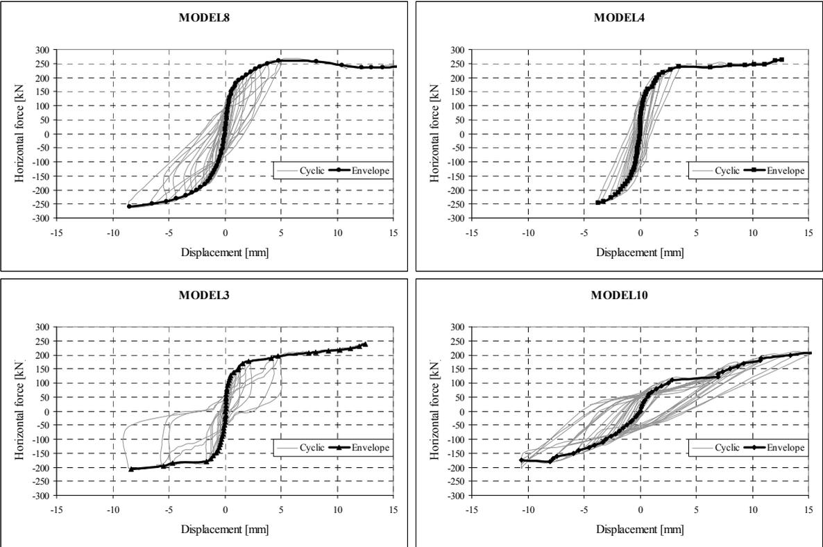
**Figure 5** Lateral load – displacement curve of the “framed-masonry” – MODEL8, 4, 3, 10
