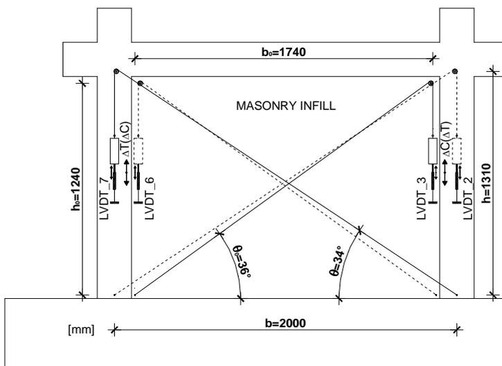
Figure 7 Shear strains measuring
