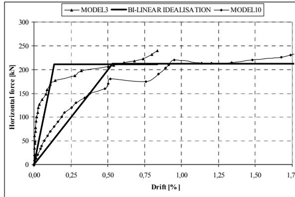
**Figure 10** Idealisation of experimental hysteretic behaviour for MODEL3
