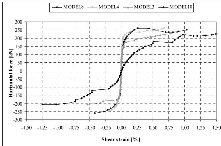
Figure 8 R/C test models' shear strain
