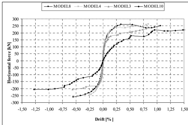
Figure 6 Test models' primary curves
