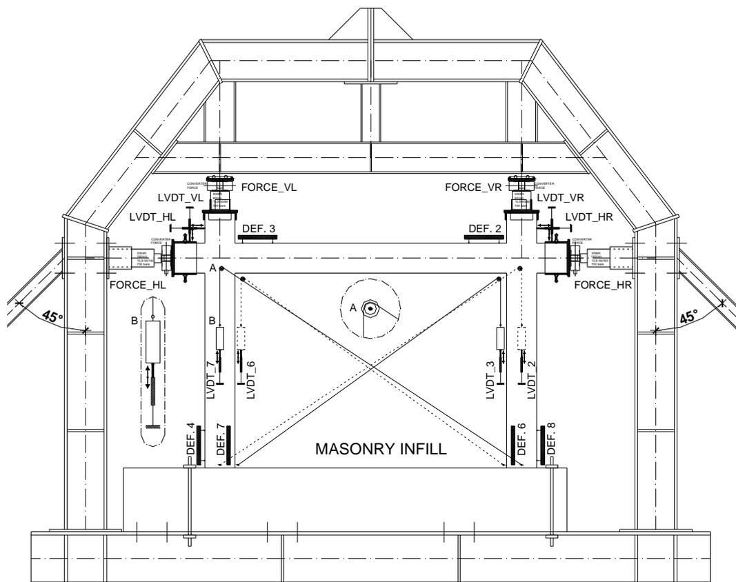
**Figure 3** Reinforced concrete infilled frame test setup
