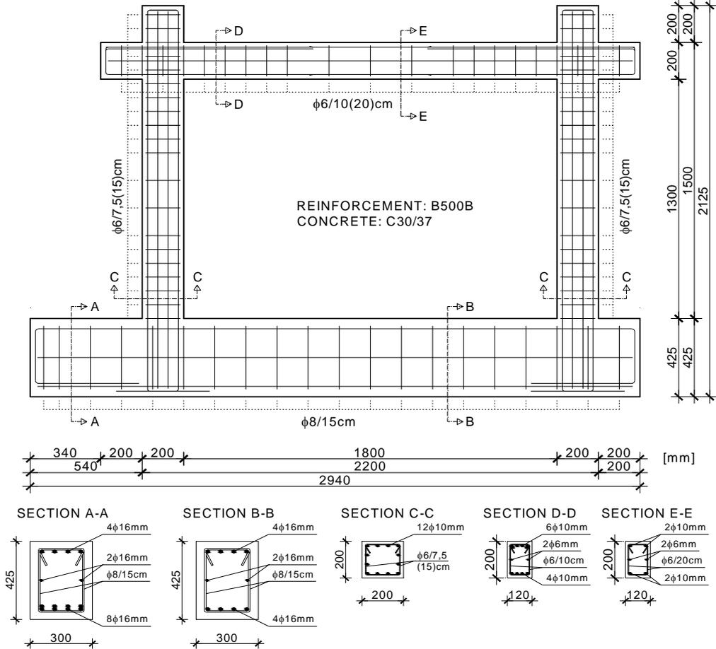
Figure 1. Dimensions and reinforcement of the test model
